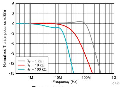
图 9-2. Bandwidth vs Frequency
