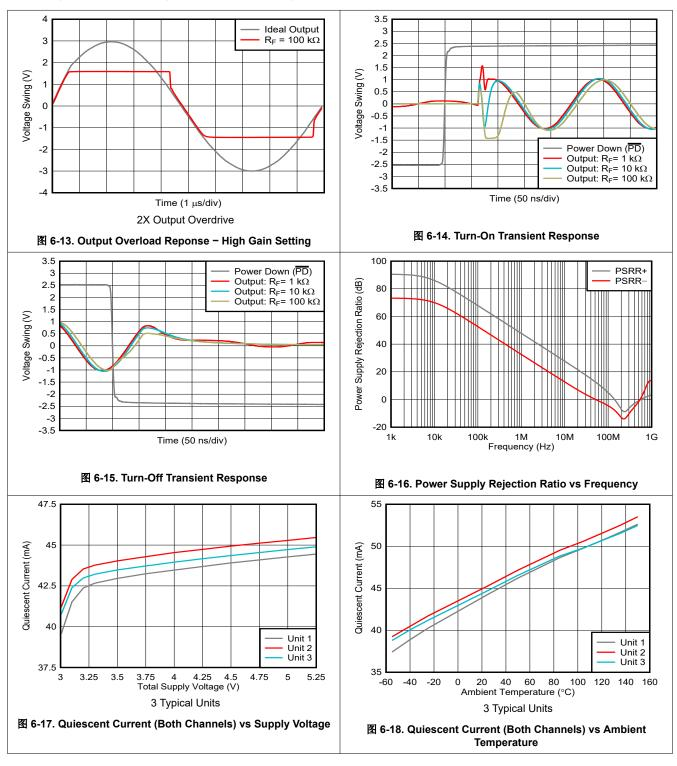
$V_{S+}$  = +2.5 V,  $V_{S-}$  = -2.5 V,  $R_L$  = 200  $\Omega$  ,  $C_{IN}$  = 4 pF, output load is referenced to mid-supply, input common-mode biased at mid-supply, and  $T_A \approx +25^{\circ}\text{C}$  (unless otherwise noted)
