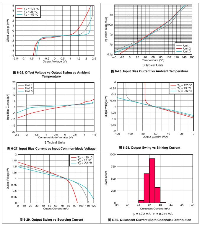
$V_{S+}$  = +2.5 V,  $V_{S-}$  = -2.5 V,  $R_L$  = 200  $\Omega$  ,  $C_{IN}$  = 4 pF, output load is referenced to mid-supply, input common-mode biased at mid-supply, and  $T_A \approx$  +25°C (unless otherwise noted)
