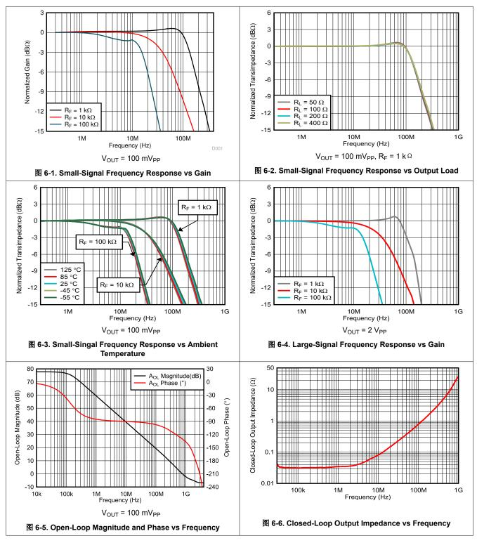
$V_{S+}$  = +2.5 V,  $V_{S-}$  = -2.5 V,  $R_L$  = 200  $\Omega$  ,  $C_{IN}$  = 4 pF, output load is referenced to mid-supply, input common-mode biased at mid-supply, and  $T_A \approx +25^{\circ}\text{C}$  (unless otherwise noted)
