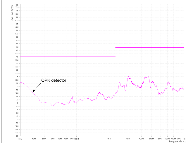
图 9-10. CISPR 32 Class B Radiated Emissions: Horizontal Polarization
