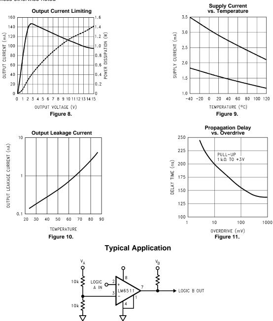
**Notes:** Because of the very wide operating and output voltage range, the LM6511 may be used to shift logic levels from 3V to TTL or CMOS to the other way around. By biasing the input to  $\frac{1}{2}$  of the input logic supply (V<sub>A</sub>), this assures that this input remains within the input voltage range. The pull-up resistor should go to the output logic supply (V<sub>B</sub>).
