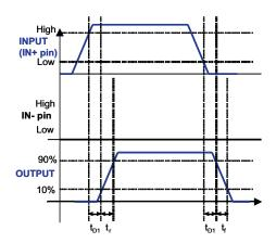
Figure 1. Non-Inverting Configuration (PWM Input to IN+ pin (IN- pin tied to GND))
