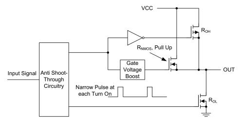
Figure 21. UCC27517A Gate Driver Output Structure
