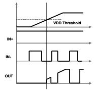
Figure 19. Power-Up (Non-Inverting Drive)
