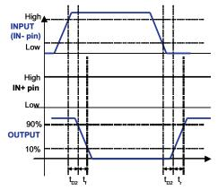
**Figure 2. Inverting Configuration** (PWM input to IN- pin (IN+ pin tied to VDD))
