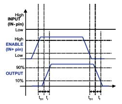
Figure 3. Enable and Disable Function Using IN+ Pin (Enable and disable signal applied to IN+ pin, PWM (Enable and disable signal applied to IN- pin, PWM input to IN- pin)
