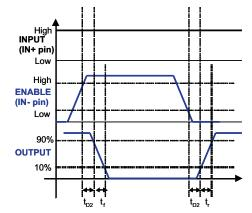
Figure 4. Enable and Disable Function Using IN-Pin input to IN+ pin)
