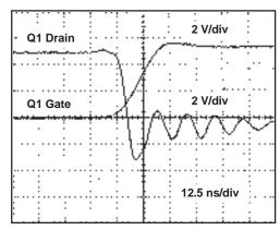
Figure 25. Q1 Turn-Off Waveform
