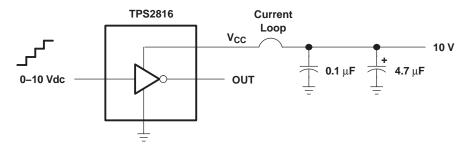
Figure 3. Shoot-Through Current Test Setup
