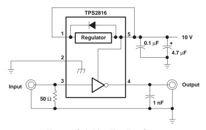
Figure 2. Switching Time Test Setup
