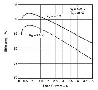
Figure 26. Converter Efficiency
