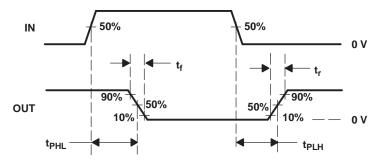
Figure 1. Typical Timing Diagram (TPS2816)
