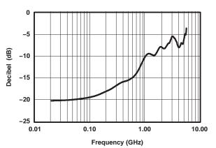
Figure 1. Differential Insertion Loss vs Frequency
