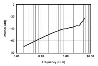
Figure 5. Differential Crosstalk vs Frequency
