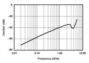
Figure 3. Common-Mode Insertion Loss vs Frequency
