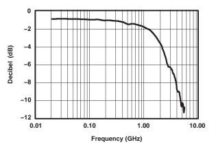
Figure 2. Differential Return Loss vs Frequency
