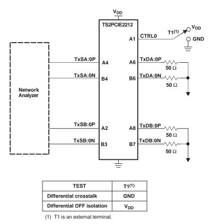
Figure 9. Differential Crosstalk and OFF Isolation Test Circuit
