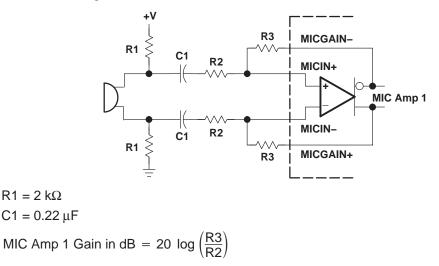
Figure 3. Typical Microphone Interface
