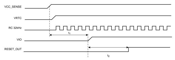
图 5-4. TPS65919-Q1 Power-Up Sequence After FSD
