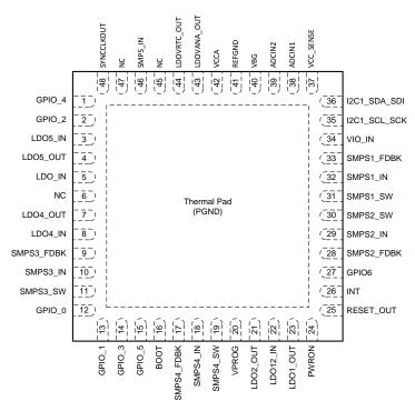
Figure 3-1. 48-Pin RGZ (VQFN) Package, 0.5-mm Pitch, With Thermal Pad (Top View)
