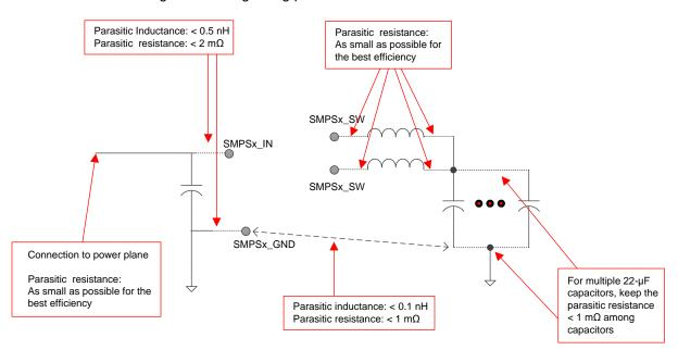
图 6-9. Parasitic Inductance and Resistance
