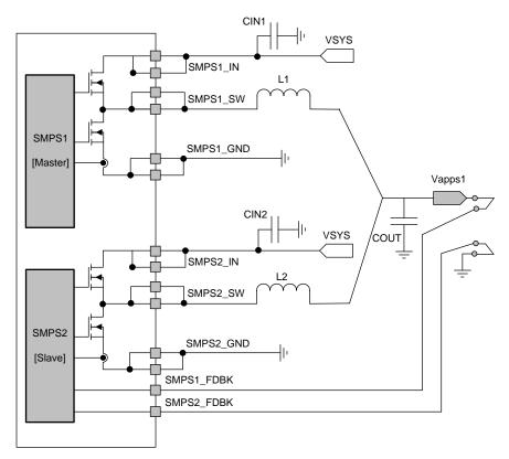
图 5-14. SMPS1&2 Dual-Phase Configuration
