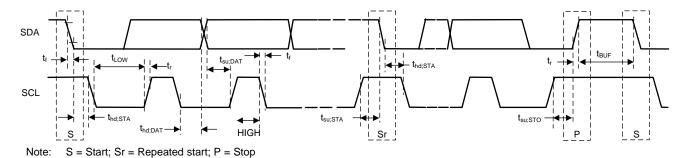
图 4-1. Serial Interface Timing Diagram For F/S Mode
