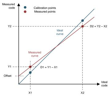
图 5-16. ADC Calibration Scheme
