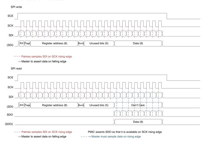
图 5-21. SPI Single Read and Write Access
