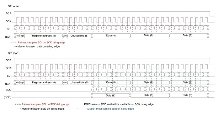
图 5-22. SPI Burst Read and Write Access
