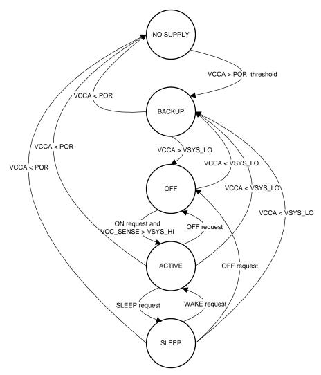
图 5-2. State Diagram for the Power Control State-Machine
