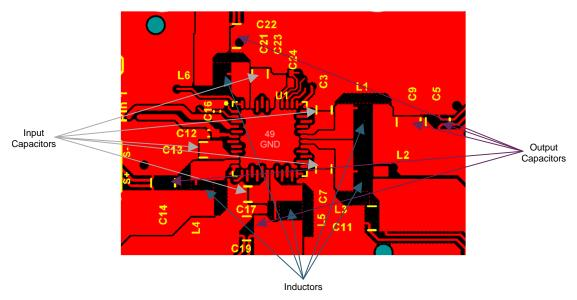
图 6-12. Top Layer Overview of Inductor and Capacitor Placement and Routing of SMPSs
