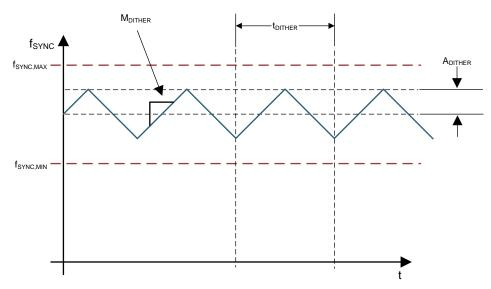
图 5-11. Synchronized Clock Frequency Range and Dither
