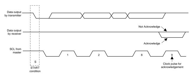
图 5-19. Acknowledge on the I<sup>2</sup>C Bus
