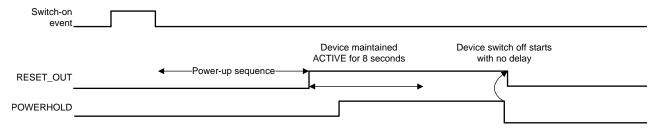
图 5-5. POWERHOLD Mode Timing Diagram
