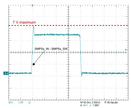
Measure across the high-side FET (SMPSx\_IN – SMPSx\_SW) as close to the IC as possible. The preferred measurement is with a differential probe. The negative side of the probe should be at SMPSx\_SW and the positive side of the probe should measure SMPSx\_IN. As shown in this image, the voltage across the high-side FET should not exceed 7 V. Repeat the measurement for all SMPSs in use.
