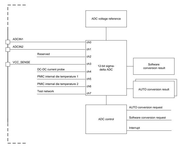
图 5-15. Block Diagram of the GPADC
