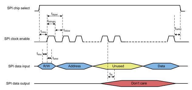
图 4-3. SPI Timings See Section 4.19 for the Timing Parameters
