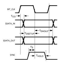
Figure 2. Data Delay, Setup and Hold
