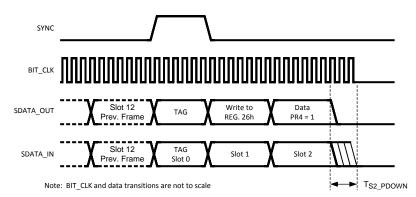
Figure 23. AC Link Power-Down Timing
