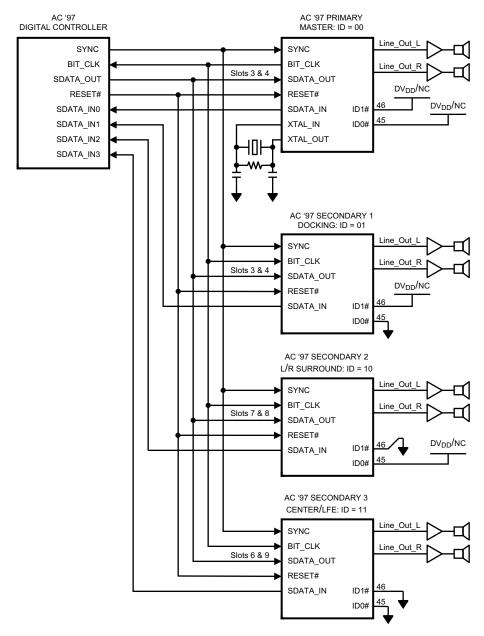
Figure 16. Multiple Codecs using Extended AC Link
