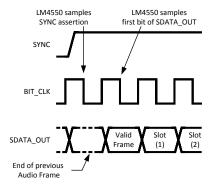
Figure 20. Start of AC Link Output Frame
