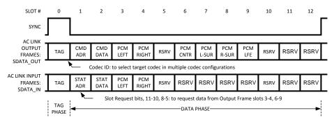
Figure 18. AC Link Bidirectional Audio Frame
