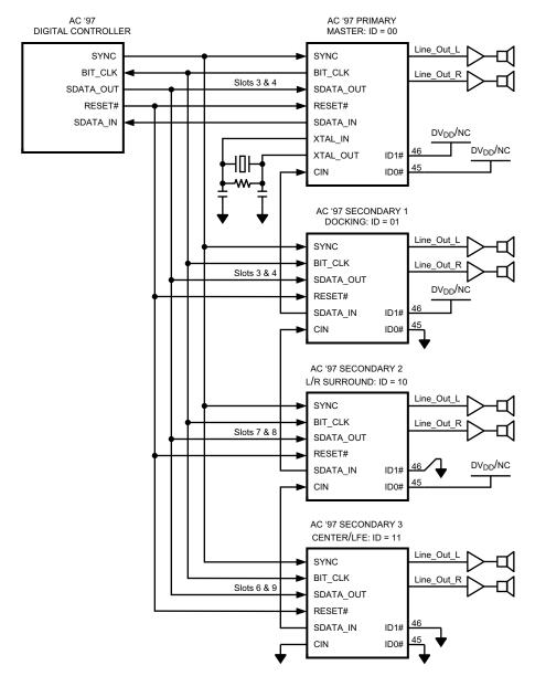
Figure 17. Multiple Codecs in a Chain
