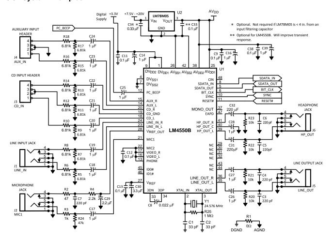
Figure 25. LM4550B Reference Design, Typical Application, Single Codec, 1 Vrms and 2 Vrms inputs, EMC output filters
