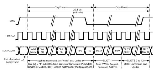
Figure 19. AC Link Output Frame
