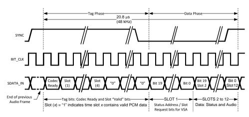
Figure 21. AC Link Input Frame
