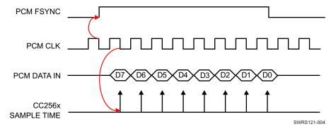
Figure 6-13. Negative Clock Edge Operation
