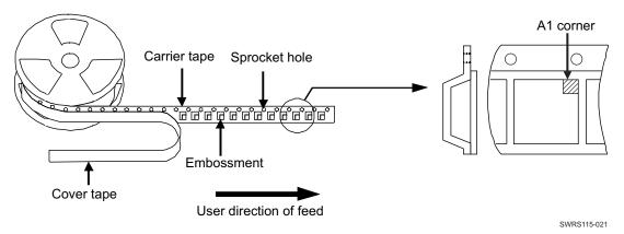
Figure 9-3. Direction of Device
