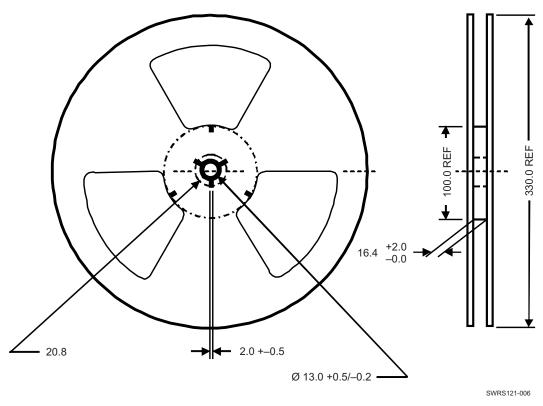
Figure 9-5. Reel Dimensions (mm)
