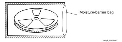
Figure 9-6. Reel Packing Method
