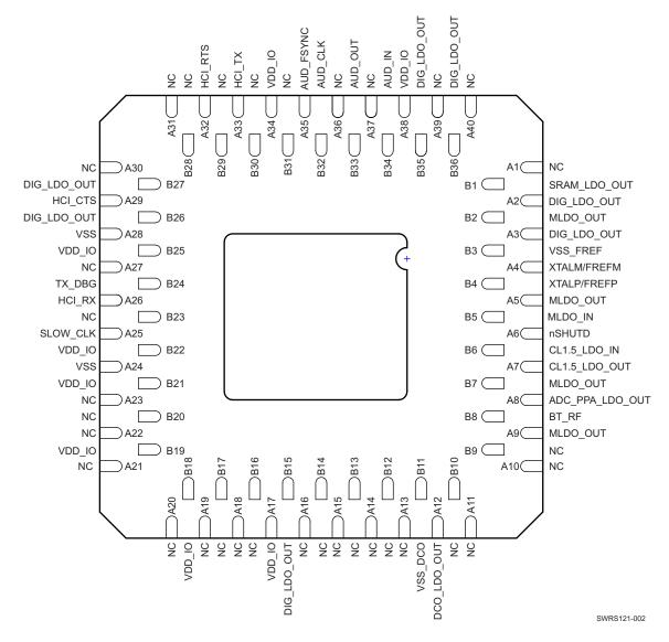
Figure 4-1. Pin Diagram (Bottom View)
