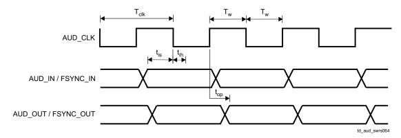
Figure 5-4. PCM Interface Timing
