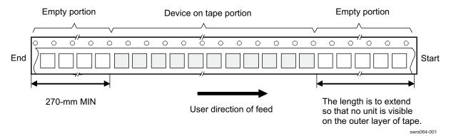
Figure 9-2. Carrier Tape and Pockets
