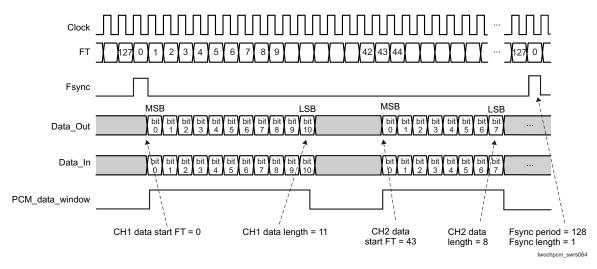
Figure 6-14. 2-Channel Bus Timing
