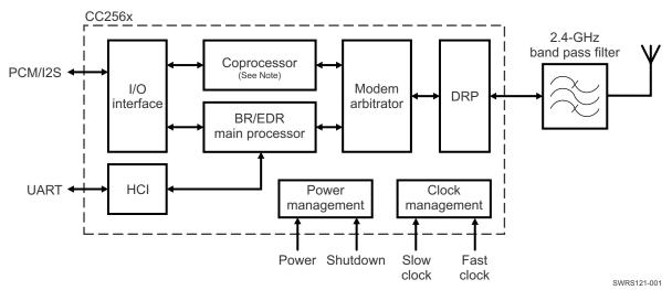
Note: The following technologies and assisted modes cannot be used simultaneously with the coprocessor: *Bluetooth* LE, ANT, assisted HFP 1.6 (WBS), and assisted A2DP. One and only one technology or assisted mode can be used at a time.
