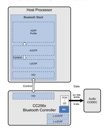
Figure 6-16. A2DP Sink Architecture Versus Assisted A2DP Sink Architecture
