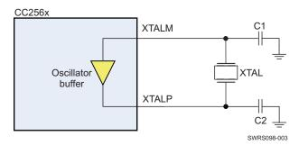
Figure 6-8. Fast-Clock Crystal Circuit
