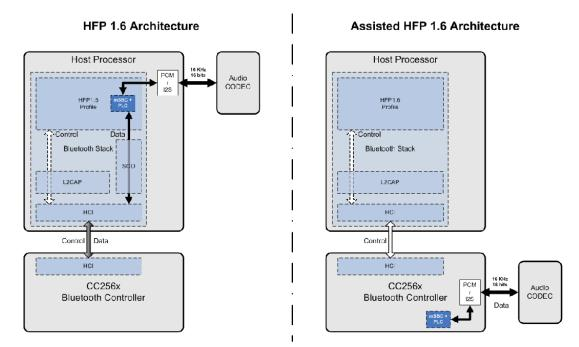
Figure 6-15. HFP 1.6 Architecture Versus Assisted HFP 1.6 Architecture
