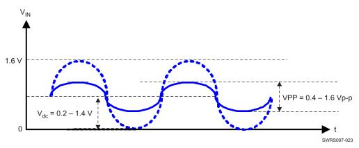
Figure 6-5. External Fast Clock (Sine Wave, DC-Coupled)
