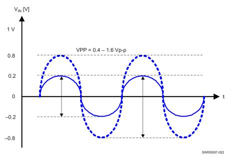
Figure 6-7. External Fast Clock (Sine Wave, AC-Coupled)
