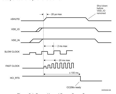
Figure 5-1. Power-Up and Power-Down Sequence
