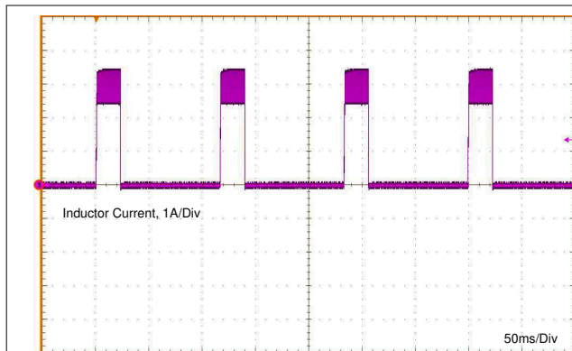
图 8-5. Inductor Current Burst in Short-Circuit Mode
