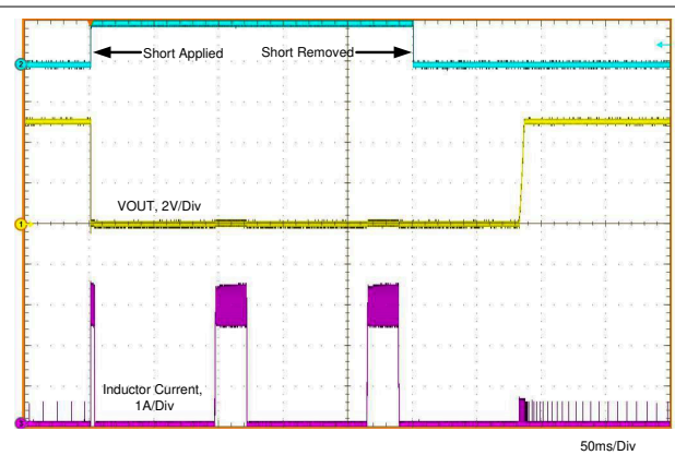
图 8-6. Short-Circuit Transient and Recovery
