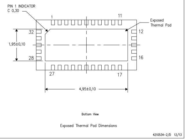
NOTE: All linear dimensions are in millimeters
