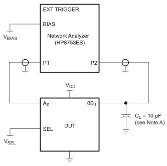
A. C<sub>L</sub> includes probe and jig capacitance.
