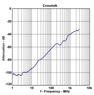
Figure 3. Crosstalk vs Frequency
