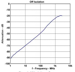
Figure 2. Off Isolation vs Frequency
