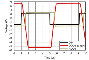
Figure 10. 250 kbps Driver to Receiver Loopback Timing Waveform,  $V_{\text{CC}}\text{=}$  3.3 V
