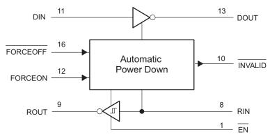
Figure 8. Logic Diagram
