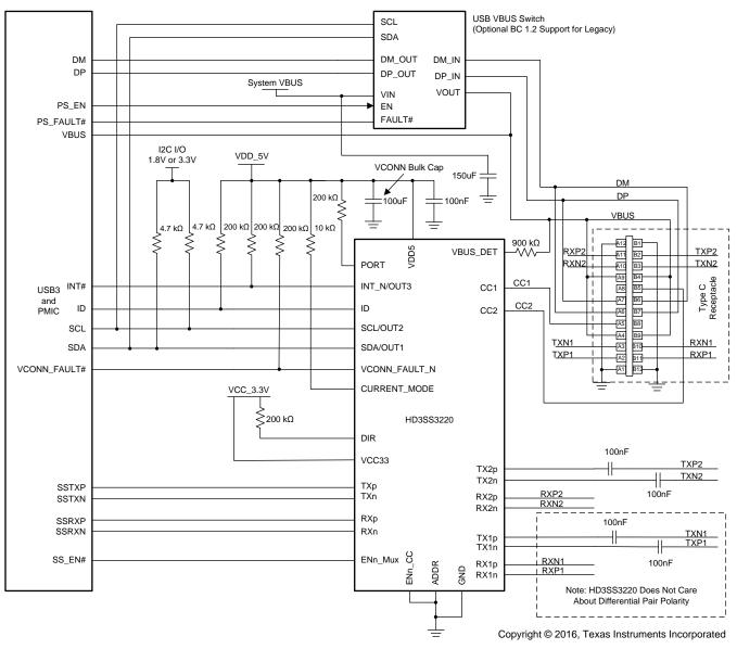
Figure 11. DFP Application Using HD3SS3220DFP
