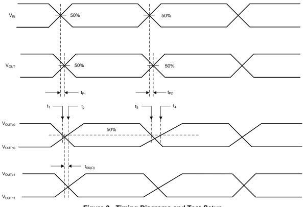
Figure 3. Timing Diagrams and Test Setup
