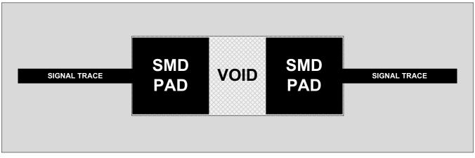
Figure 20. Reference Plane Voiding of Surface-Mount Devices
