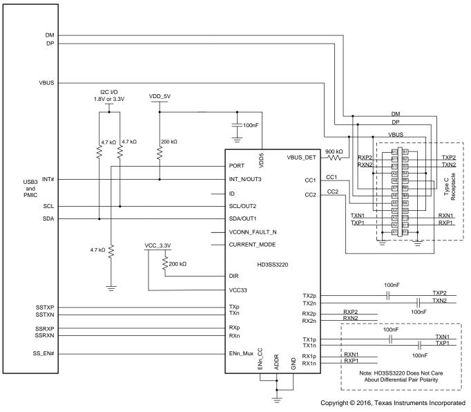
Figure 12. UFP Application Using HD3SS3220DFP
