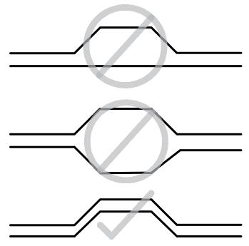
Figure 16. Differential Pair Symmetry
