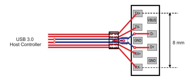
Figure 21. Flow-Through Routing
