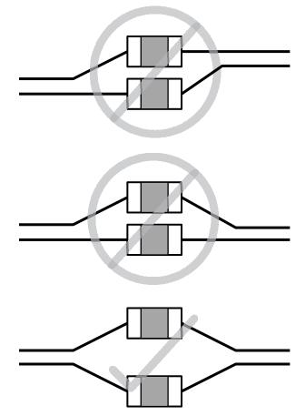
Figure 19. AC-Coupling Placement
