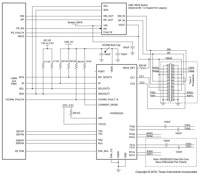
Figure 10. DRP Application Using HD3SS3220DRP
