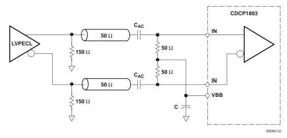
Figure 9. Recommended AC-Coupling LVPECL Receiver Input Termination
