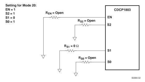
Figure 1. Control Terminal Setting for Example
