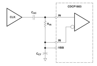
NOTE: C<sub>AC</sub> - AC-coupling capacitor (e.g., 10 nF)
