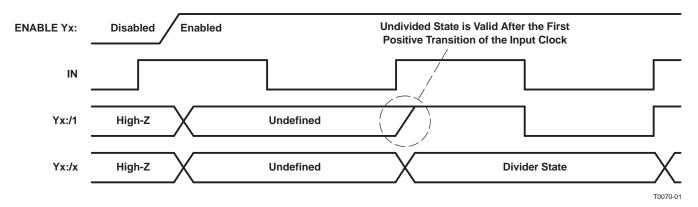
Figure 14. Signal State After an Output Driver Becomes Enabled While IN = 1
