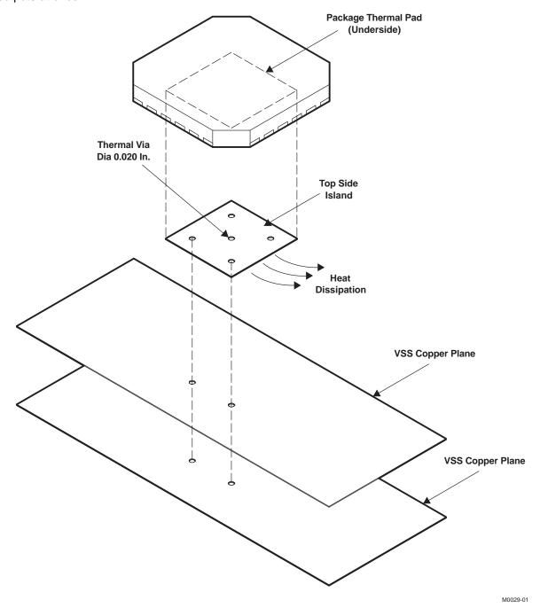
Figure 8. Recommended Thermal Via Placement
