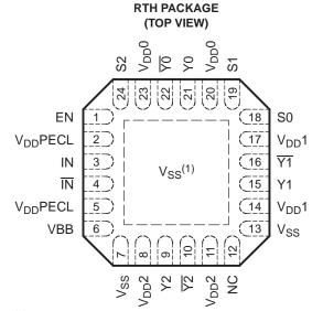
(1) Thermal pad must be connected to V<sub>SS</sub>.
