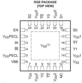
(1) Thermal pad must be connected to V<sub>SS</sub>.
