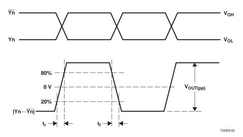
Figure 7. LVPECL Differential Output Voltage and Rise/Fall Time
