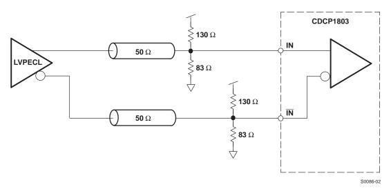
Figure 10. Recommended DC-Coupling LVPECL Receiver Input Termination
