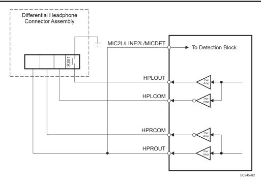
图 9-10. Configuration of Device for Jack Detection Using Fully-Differential Stereo Headphone Output Connection
