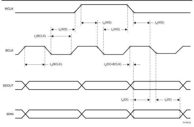
图 8-4. DSP Timing in Slave Mode
