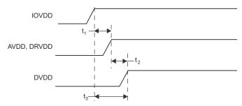
图 11-1. Power-Supply Sequencing
