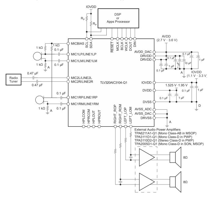
图 10-1. Typical Connections With Differential Inputs for External Speaker Driver
