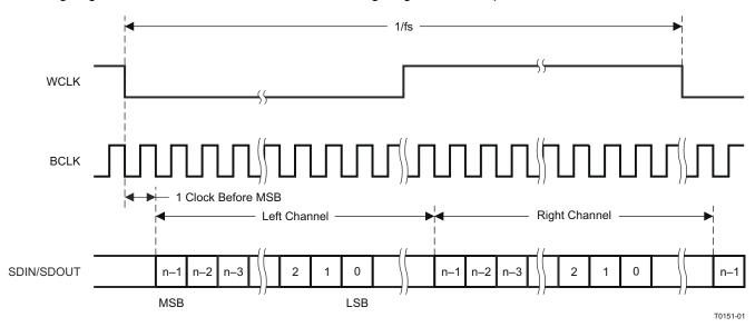
图 9-18. I<sup>2</sup>S Serial Data Bus Mode Operation
