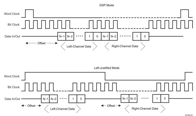
图 9-20. DSP Mode and Left-Justified Mode, Showing the Effect of a Programmed Data-Word Offset
