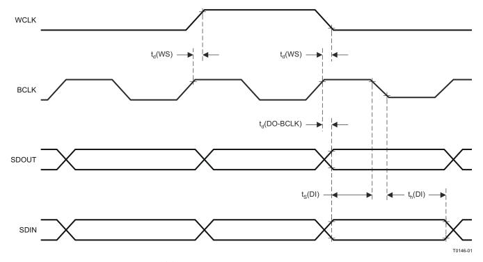
图 8-3. DSP Timing in Master Mode
