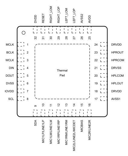
NOTE: Connect the device thermal pad to DRVSS.
