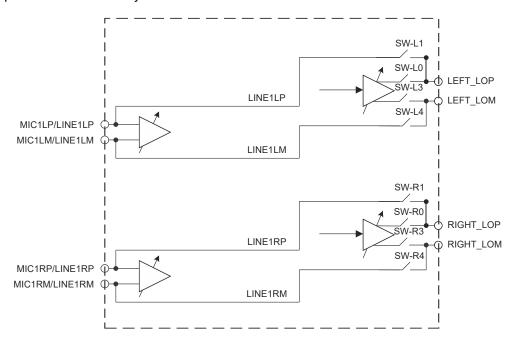
图 9-12. Passive Analog Bypass Mode Configuration
