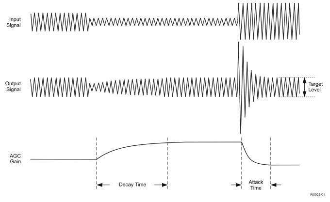
图 9-1. Typical Operation of the AGC Algorithm During Speech Recording
