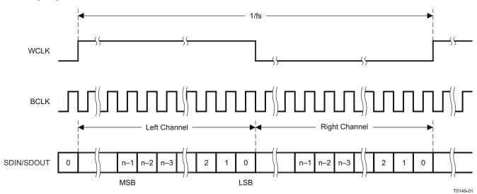
图 9-16. Right-Justified Serial Data Bus Mode Operation
