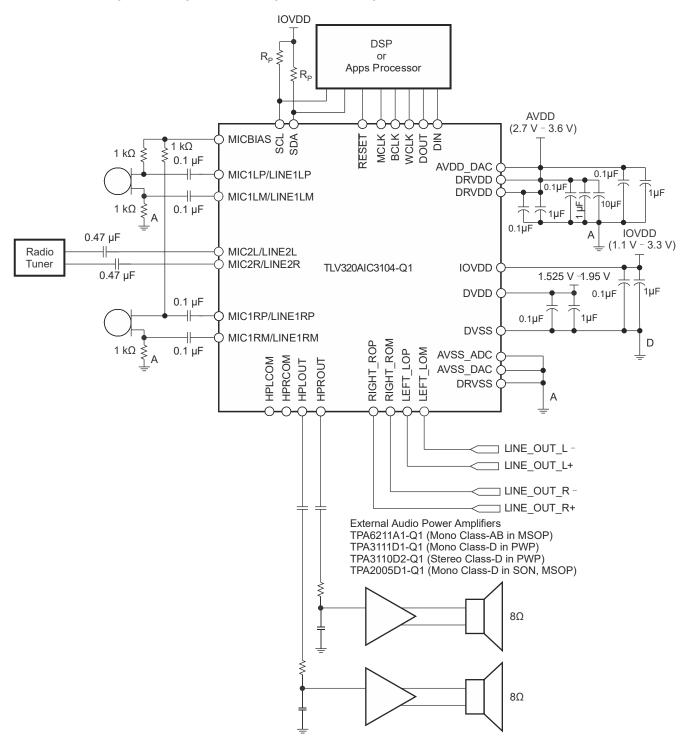
图 10-5. Typical Connections With Single-Ended Outputs for External Amplifier With Separate Line Outputs
