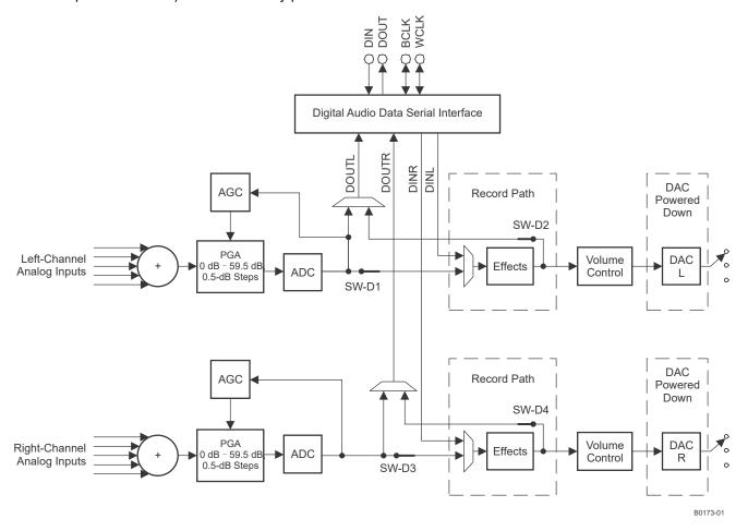
图 9-11. Record-Only Mode With Digital Processing Path Enabled
