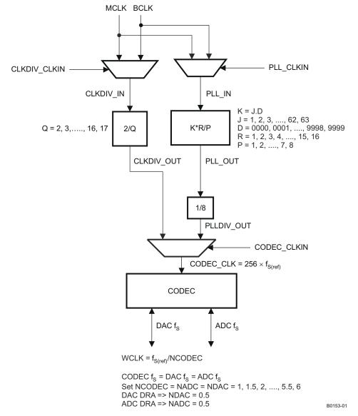
图 9-21. Audio Clock Generation Processing
