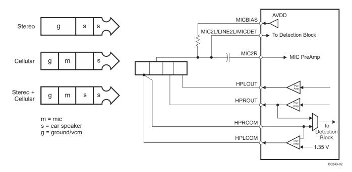
图 9-8. Configuration of Device for Jack Detection Using Pseudo-Differential (Capless) Headphone Output Connection
