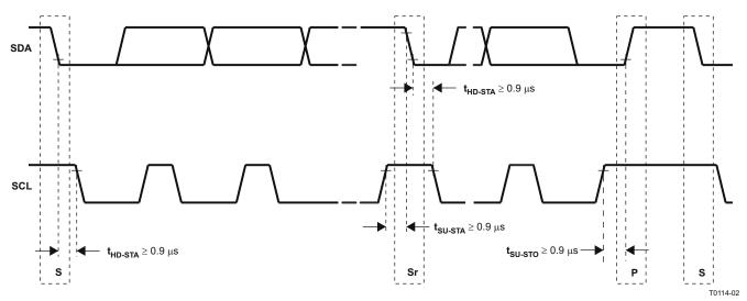
图 9-13. I<sup>2</sup>C Interface Timing
