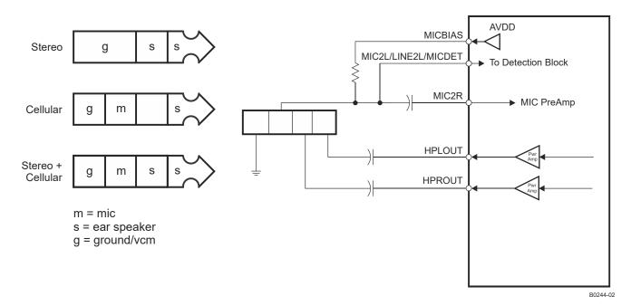
图 9-9. Configuration of Device for Jack Detection Using AC-Coupled Stereo Headphone Output Connection
