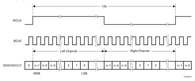
图 9-17. Left-Justified Serial Data Bus Mode Operation
