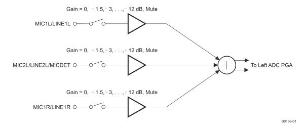
图 9-4. Single-Ended Analog Input Mixing Configuration
