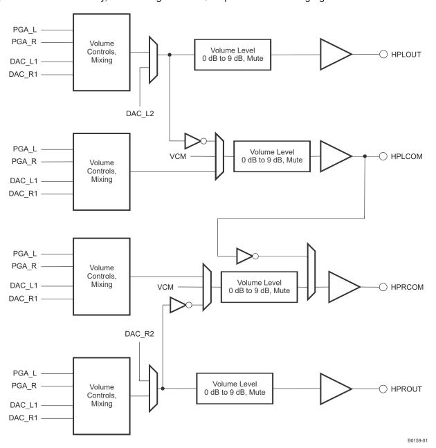
图 9-7. Architecture of Output Stage Leading to High-Power Output Drivers
