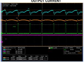
Figure 20. f = 800kHz,  $V_{IN}$  = 20V,  $I_{OUT}$  = 8A
