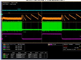
Figure 22. f = 800kHz,  $V_{IN} = 20V$ ,  $I_{OUT} = 0-6A$
