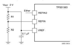
Figure 28. Setting the Output Voltage
