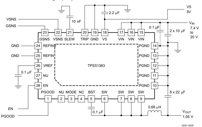
Figure 32. Design 1: Application Schematic
