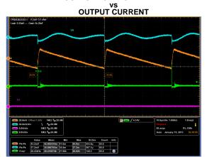
Figure 19. f = 800kHz,  $V_{IN}$  = 20V,  $I_{OUT}$  = 0.1A
