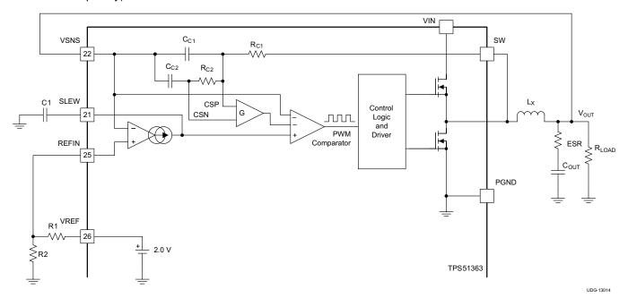
Figure 30. Simplified Architecture Illustrating DCAP2 Mode
