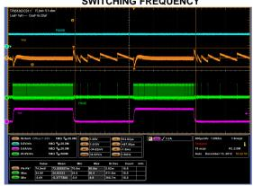
Figure 21. f = 400kHz,  $V_{IN} = 20V$ ,  $I_{OUT} = 0-5A$
