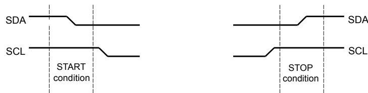
Figure 18-3. START and STOP Conditions
