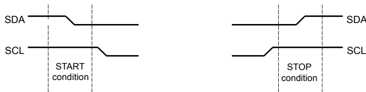
Figure 14-3. START and STOP Conditions
