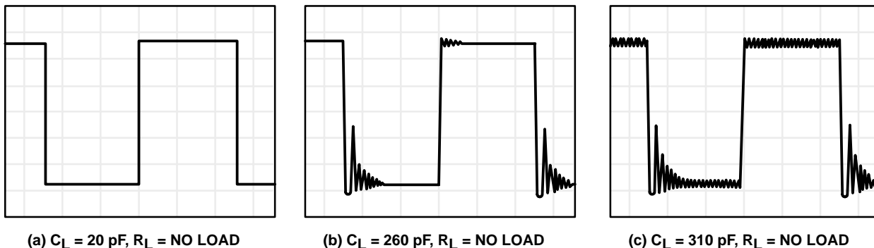
Figure 112. Effect of Capacitive Loads in Low-Bias Mode
