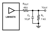
Figure 32. Decoupling Capacitive Loads
