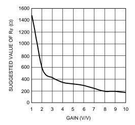
Figure 26. Suggested R<sub>F</sub> vs. Gain
