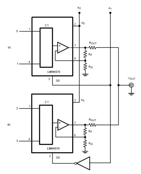
Figure 27. 4:1 MUX Using Two LMH6570 Devices
