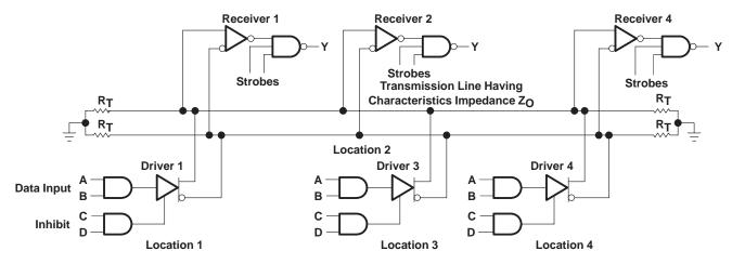
Receivers are SN75207B; drivers are SN55109A, SN55110A, SN75110A, or SN75112.
