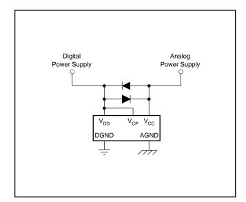
FIGURE 15. Latch-up Prevention Circuit.
