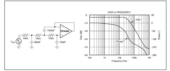
FIGURE 12. 3rd-Order Low-Pass Filter.
