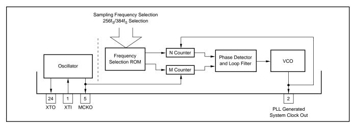
FIGURE 2. PLL Block Diagram.
