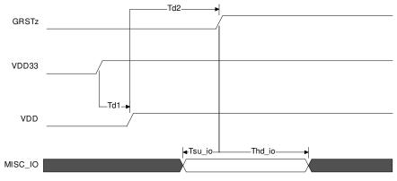
图 7-1. Power-Up Timing Requirements
