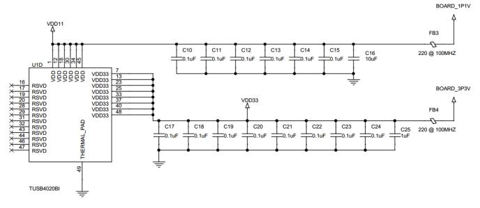
图 9-10. Power Implementation Schematic
