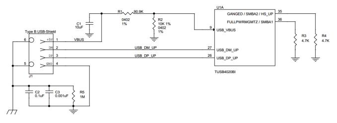
图 9-3. Upstream Port Implementation Schematic
