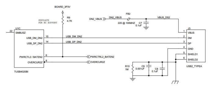
图 9-7. Downstream Port 2 Implementation Schematic
