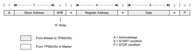
Figure 49. "Write" Data Transfer Format in F/S-Mode
