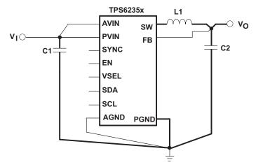
Figure 53. Layout Diagram
