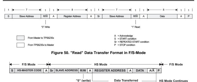
Figure 51. Data Transfer Format in H/S-Mode
