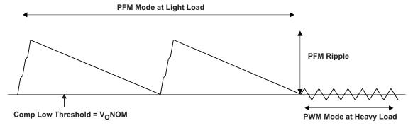
Figure 44. Operation in PFM Mode and Transfer to PWM Mode
