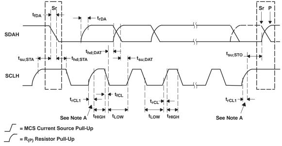
Note A: First rising edge of the SCLH signal after Sr and after each acknowledge bit.
