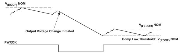
Figure 52. PWROK Operation (Transition to a Lower Voltage)
