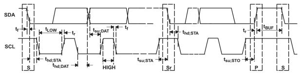
Figure 1. Serial Interface Timing Diagram for F/S-Mode
