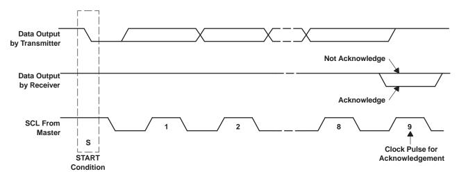
Figure 47. Acknowledge on the I<sup>2</sup>C Bus
