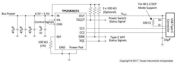
图 19. Type-C Source Port Implementation with BC 1.2 (DCP Mode) Support
