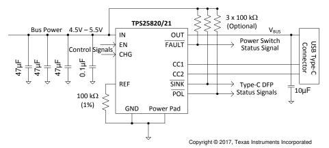
图 12. Type-C Source Port Implementation without BC 1.2 Support
