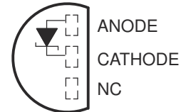
1.2 V ... LP (TO-92/TO-226) PACKAGE (TOP VIEW)
