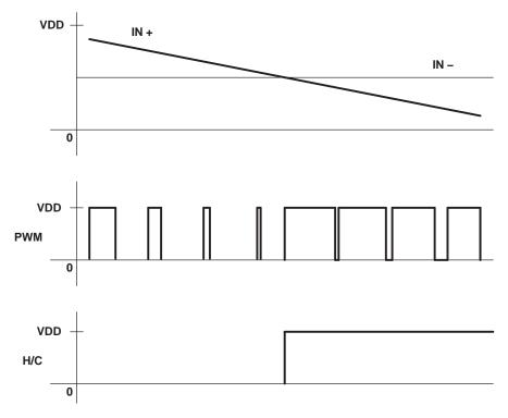
Figure 20. Transition From Cooling to Heating
