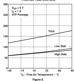
$r_{DS(on)}$  – Drain-Source On-State Resistance –  $m\Omega$
