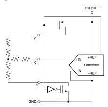
Figure 25. Simplified Diagram of Single-Ended Reference
