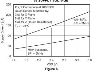
SUPPLY CURRENT (Part Not Addressed) vs SUPPLY VOLTAGE
