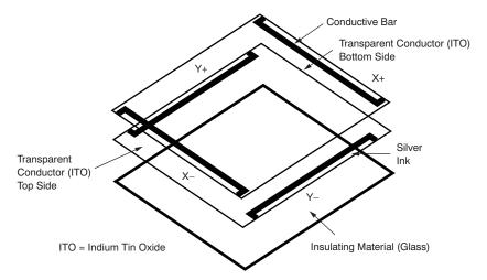
Figure 21. 4-Wire Touch Screen Construction
