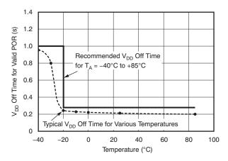
Figure 38. V<sub>DD</sub> Off Time vs Temperature
