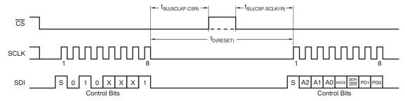
Figure 35. Software Reset Timing
