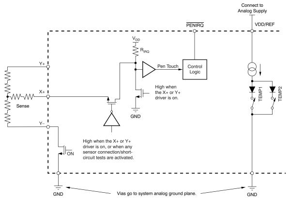
Figure 27. Example of a Pen-Touch Induced Interrupt via the PENIRQ Pin
