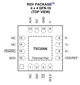
(1) The thermal pad is internally connected to the substrate. The thermal pad can be connected to the analog ground or left floating. Keep the thermal pad separate from the digital ground, if possible.
