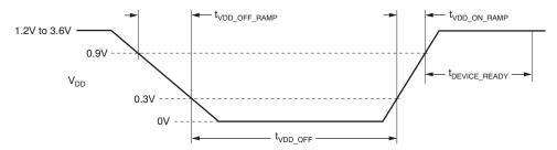
Figure 37. Power-On Reset Timing
