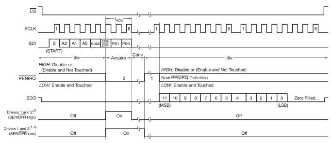
NOTES: (1) For Y-Position, Driver 1 is on X+ is selected, and Driver 2 is off. For X-Position, Driver 1 is off, Y+ is selected, and Driver 2 is on. Y- will turn on when power-down mode is entered and PD0 = 0.
