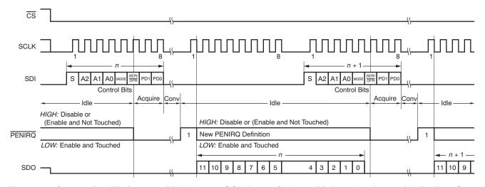
Figure 31. Conversion Timing—12-Bit Mode, 16 SCLKs per Cycle, 8-Bit Bus Interface, with Earliest Start of New Command
