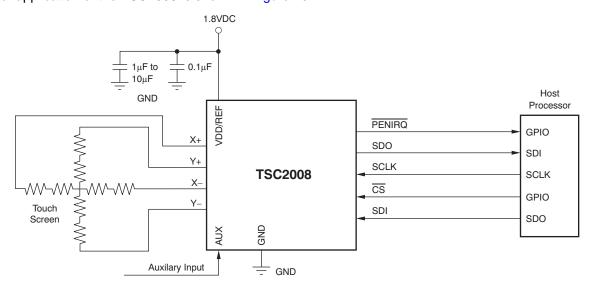
Figure 20. Typical Circuit Configuration
