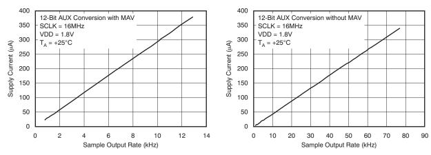
Figure 34. Sample Output Rate vs Supply Current (with and without MAV filter)
