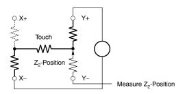
Figure 22. Pressure Measurement
