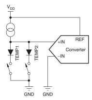
Figure 23. Functional Block Diagram of Temperature Measurement Mode
