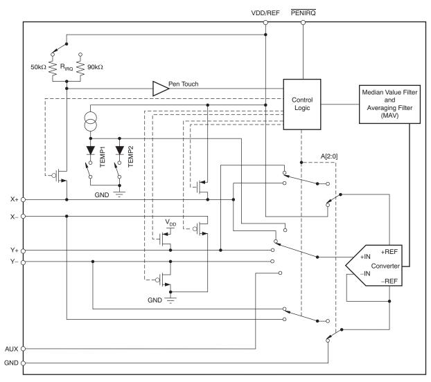
Figure 24. Analog Input Section (Simplified Diagram)
