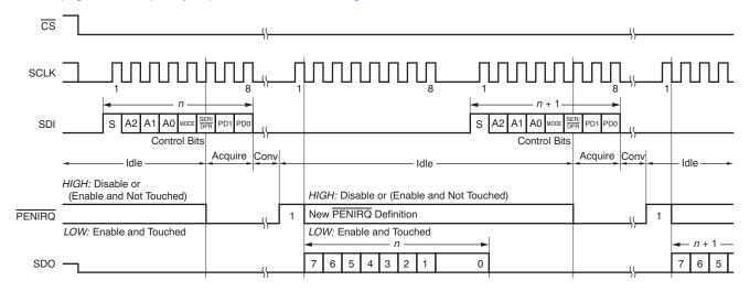
Figure 32. Conversion Timing—8-Bit Mode, 16 SCLKs per Cycle, 8-Bit Bus Interface, without Adjusted SDO Timing (TSC2046-Compatible)
