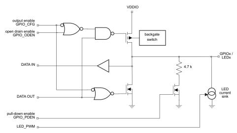
Figure 7-2. GPIO Block for GPIO3, GPIO4, and GPIO5
