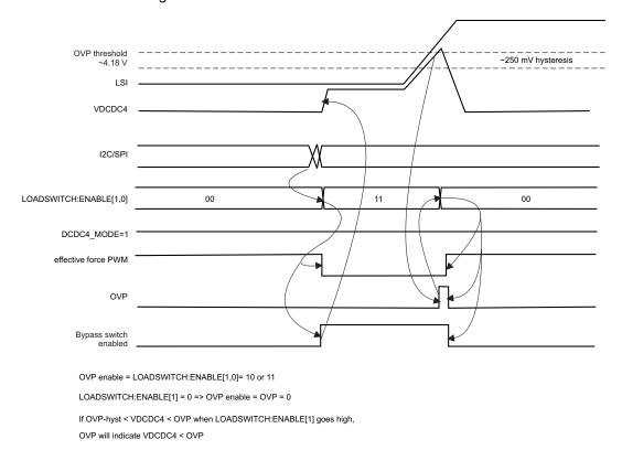
Figure 7-28. Load Switch Timing for LOADSWITCH:ENABLE[1,0] = 10 or 11
