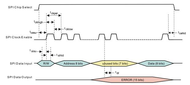
Figure 6-3. SPI Interface Timing
