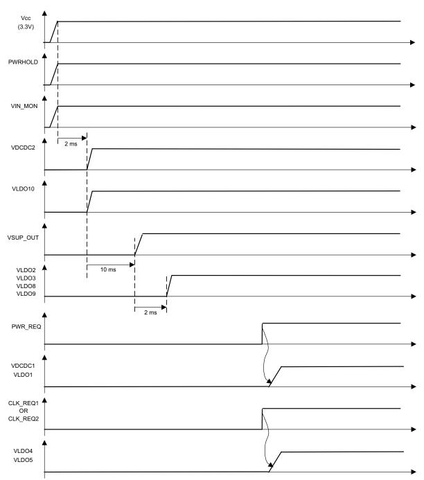
Figure 7-14. TPS659121 3.3-V Host Power Up With CONFIG1=LOW
