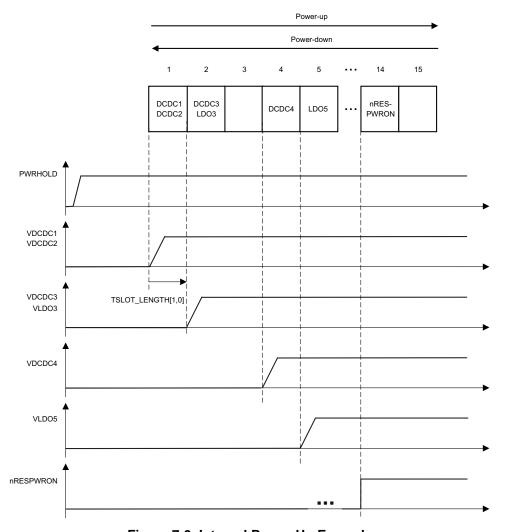
Figure 7-9. Internal Power-Up Example
