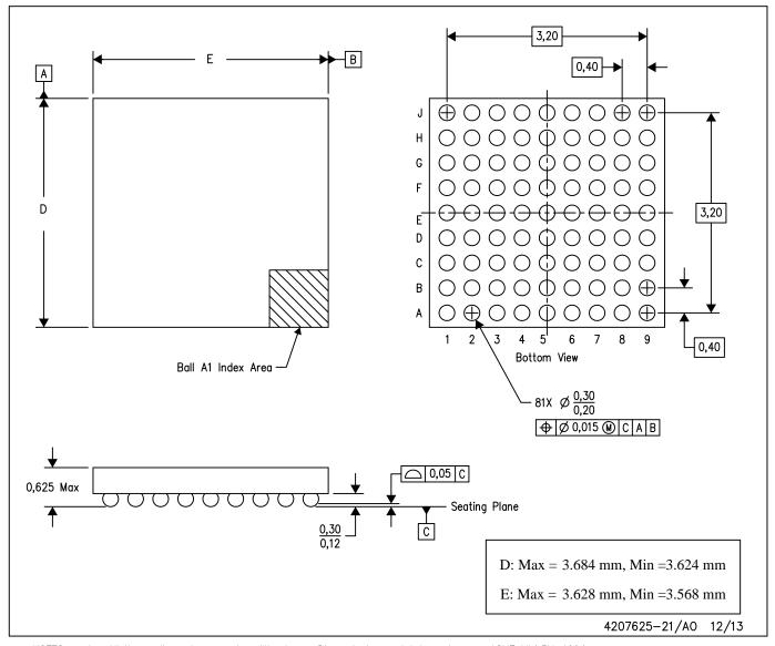
NOTES: A. All linear dimensions are in millimeters. Dimensioning and tolerancing per ASME Y14.5M-1994.
