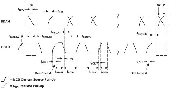
A. First rising edge of the SCLH signal after Sr and after each acknowledge bit.
