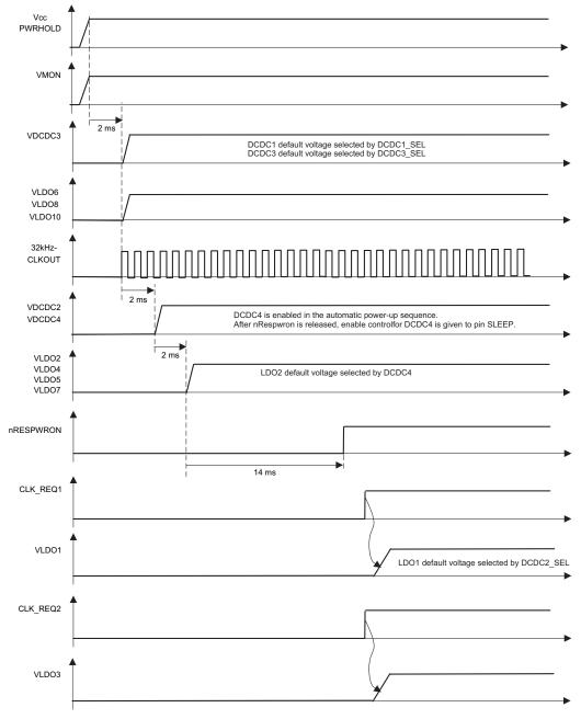
Figure 7-15. TPS659122 Power Up With CONFIG1=HIGH
