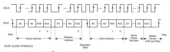
Figure 7-25. I<sup>2</sup>C Interface READ from TPS65912x; F/S mode
