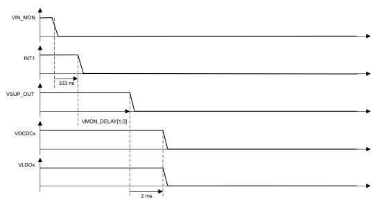
Figure 7-16. TPS659121, TPS659122 Power Cut With CONFIG1=HIGH
