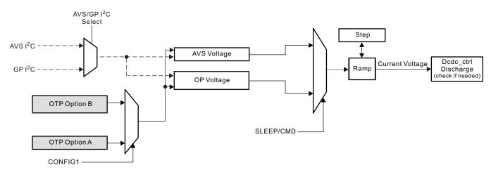
Figure 7-11. DC-DC Voltage Scaling Architecture
