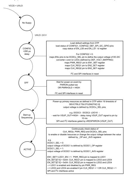
Figure 7-5. STARTUP Flow for CONFIG2=0
