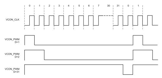
Figure 7-12. VCON Voltage Scaling Architecture
