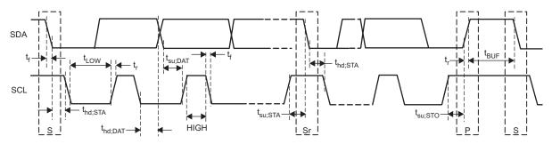
Figure 6-1. Serial Interface Timing Diagram for FS-Mode
