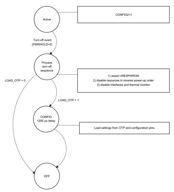
Figure 7-7. SHUTDOWN Flow for CONFIG2=1
