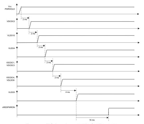
Figure 7-17. TPS659122 Power Up With CONFIG1=LOW
