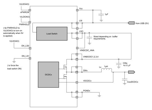
Figure 7-26. Load Switch Connected as USB Input Current Limited Switch
