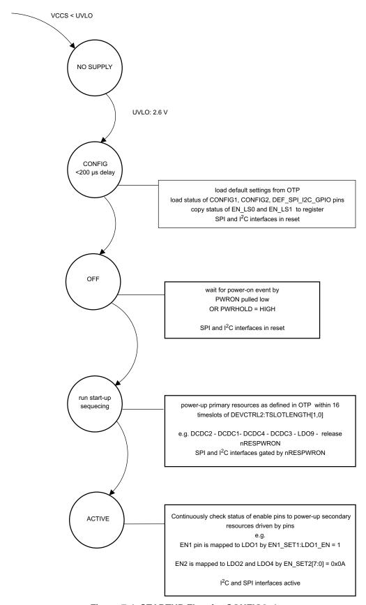
Figure 7-4. STARTUP Flow for CONFIG2=1
