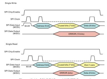
Figure 7-18. SPI READ and WRITE Protocol
