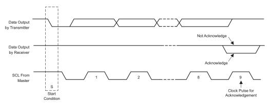
Figure 7-22. Acknowledge on the I<sup>2</sup>C Bus
