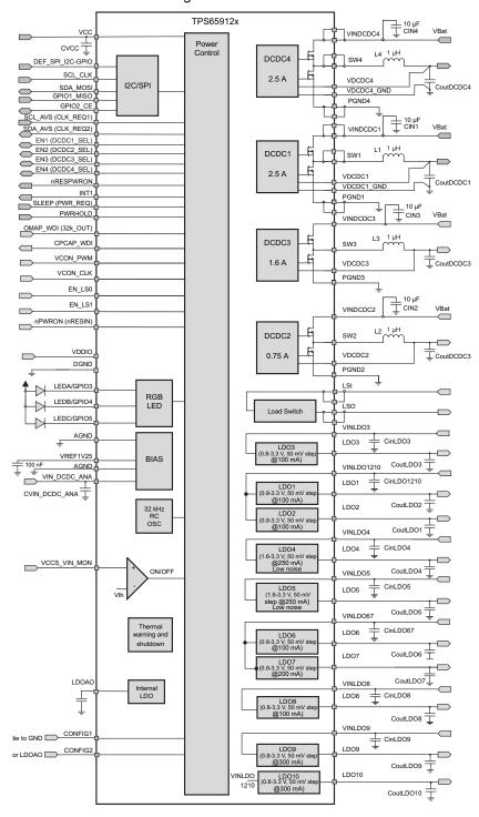
Figure 1-1. TPS65912x Block Diagram
