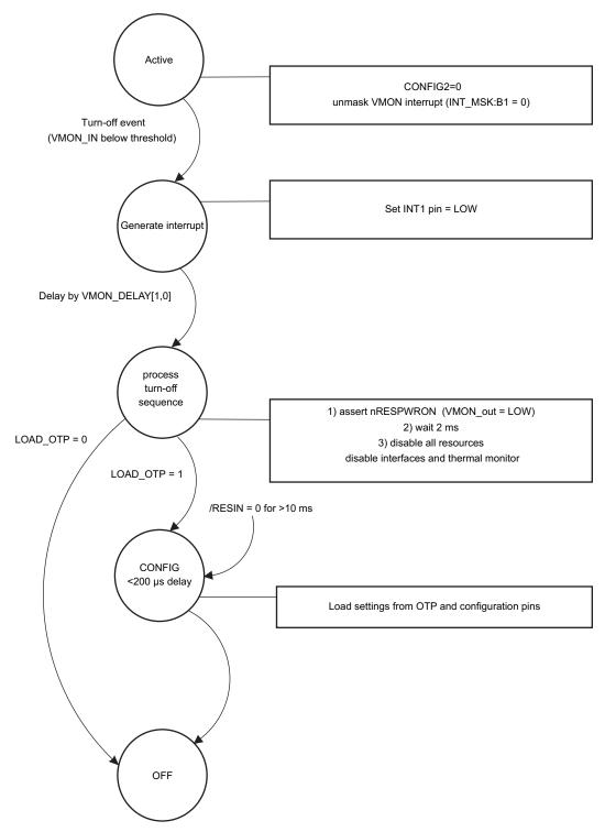
Figure 7-8. SHUTDOWN Flow for CONFIG2=0
