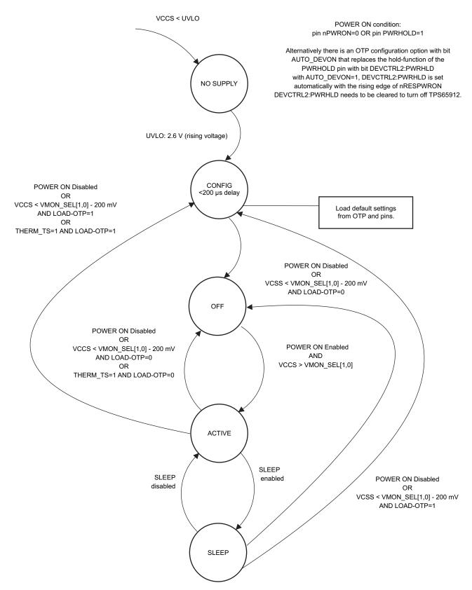
Figure 7-3. Embedded Power Control State Machine
