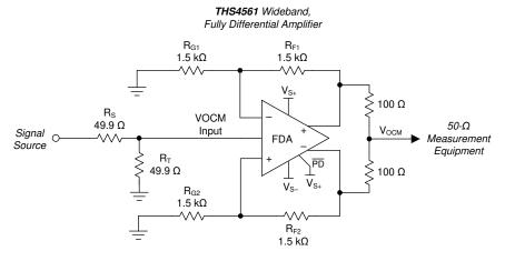
图 8-5. Output Common-Mode Measurements
