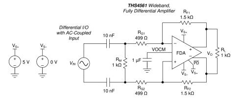
图 9-1. Example AC-Coupled Differential Input Design
