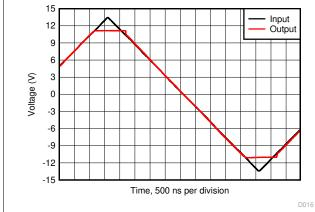
V<sub>S</sub> = 12 V, Single-ended to differential gain of 2, 2-V output overdrive,
