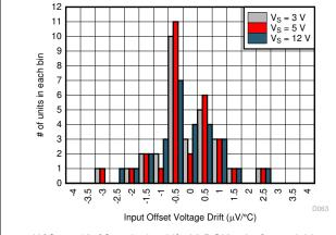
– 40°C to +125°C endpoint drift, 30 DGK units for each  $V_{\mbox{\scriptsize S}}$
