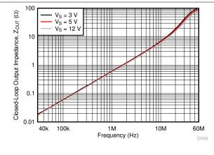
图 7-43. Closed-Loop Output Impedance vs Frequency
