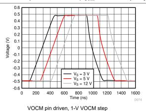
图 7-50. Common-Mode Voltage Large-Signal Step Response
