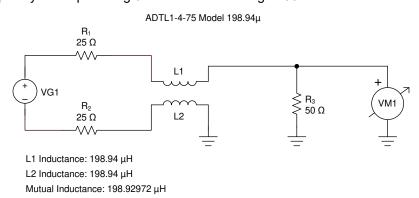
图 8-2. Output Measurement Balun Simulation Circuit in TINA-TI™
