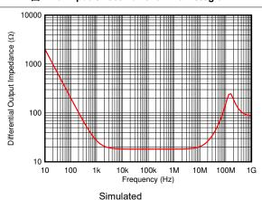
图 7-42. Open-Loop Output Impedance vs Frequency
