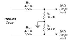
图 8-4. Output Interface for DC-Coupled Differential Outputs
