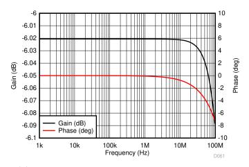
图 8-3. Output Measurement Balun Flatness Test
