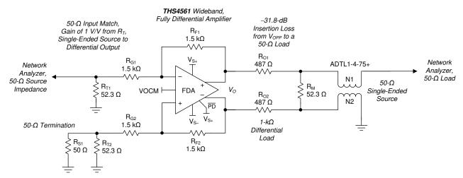
图 8-1. Single-Ended Source to a Differential Gain of a 1-V/V Test Circuit
