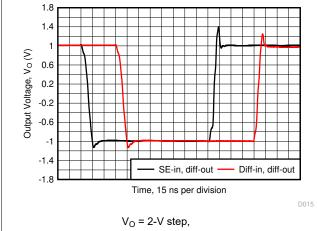
$V_O=2\text{-V step},$  SE-in, diff-out: rising SR = 350 V/ $\mu$ s, falling SR = 200 V/ $\mu$ s, diff-in, diff-out: rising SR = 285 V/ $\mu$ s, falling SR = 285 V/ $\mu$ s
