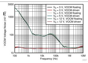
The VOCM pin is either driven to midsupply by low-impedance source or allowed to float and default to midsupply
