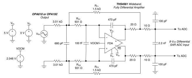
图 10-7. MFB Filter Driving an ADC Application: Example 170-kHz Butterworth Response
