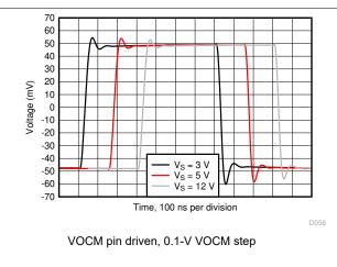
图 7-49. Common-Mode Voltage Small-Signal Step Response
