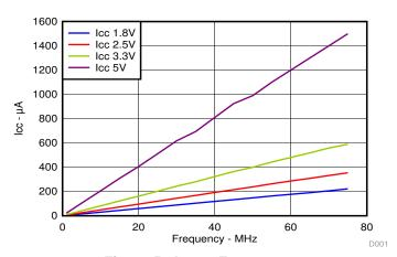
Figure 5. I<sub>CC</sub> vs Frequency
