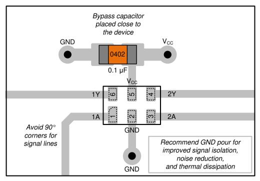
Figure 6. Layout example for DRY package
