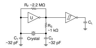
Figure 4. Typical Application Diagram
