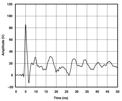
Figure 6. IEC ESD Clamping Waveforms +8-KV Contact
