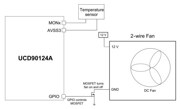
Figure 25. Two-Wire Fan Connection
