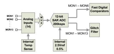
Figure 12. Voltage Monitoring Block Diagram
