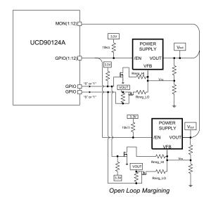
Figure 23. Open-Loop Margining
