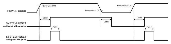
Figure 30. System Reset with and without Pulse Setting
