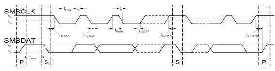
Figure 1. I<sup>2</sup>C/SMBus Timing Diagram
