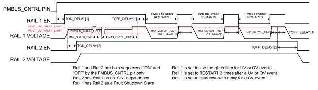
Figure 16. Sequencing and Fault-Response Timing
