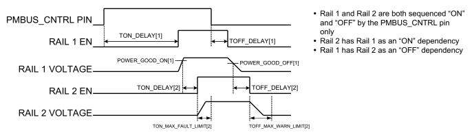
Figure 11. Sequence-on and Sequence-off Timing
