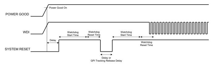
Figure 31. System Reset with Watchdog
