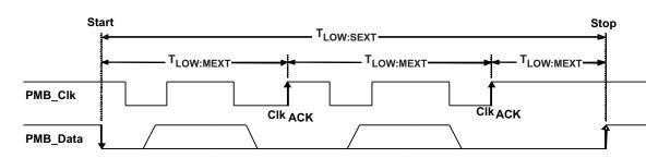
Figure 2. Bus Timing in Extended Mode
