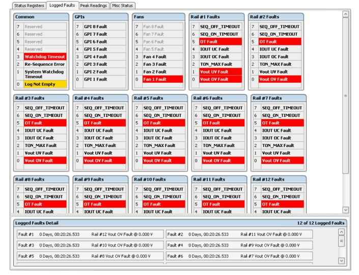
Figure 10. Fusion GUI Flash-Error Log (Logged Faults)
