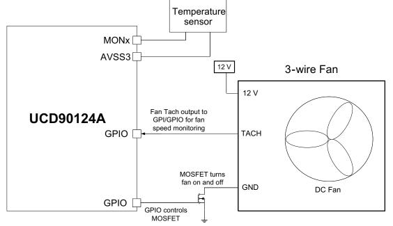
Figure 26. Three-Wire Fan Connection
