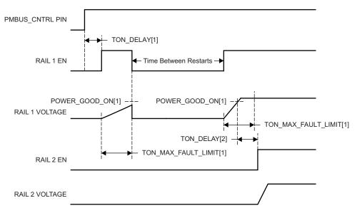
Rail 1 and Rail 2 are both sequenced "ON" and "OFF" by the PMBUS\_CNTRL pin only
