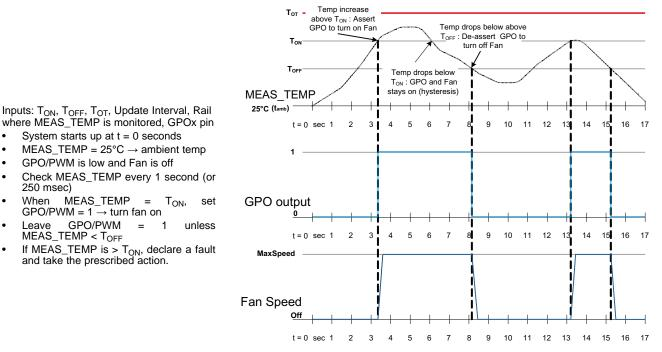
Figure 28. Hysteretic Temperature Control for 2- or 3-wire Fans
