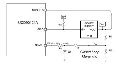
Figure 24. Closed-Loop Margining
