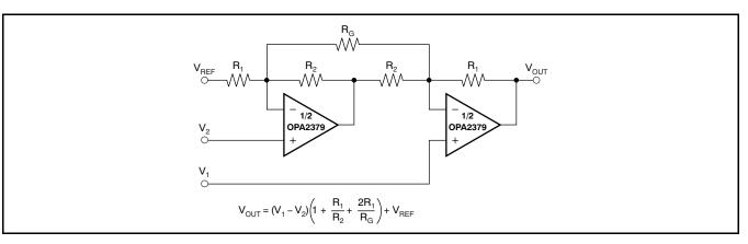
Figure 29. Two Op Amp Instrumentation Amplifier
