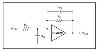
Figure 22. Improving Stability for Large  $R_{\rm F}$  and  $R_{\rm IN}$
