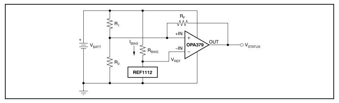
Figure 23. Battery Monitor
