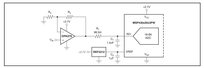
Figure 25. Unipolar Signal Chain Configuration
