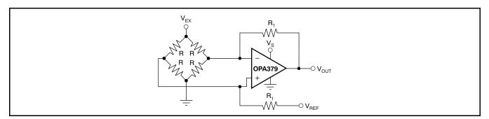
Figure 26. Single Op Amp Bridge Amplifier
