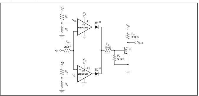
(1)  $R_{\text{IN}}$  protects A1 and A2 from possible excess current flow.
