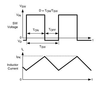
Figure 13. Typical Waveforms
