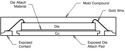
Figure 25. Internal WSON Connection
