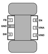
Figure 24. 6-Lead WSON PCB Dog-Bone Layout
