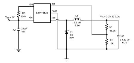
Figure 21. LMR10520X (1.6 MHz):  $V_{IN}$  = 5 V,  $V_{OUT}$  = 3.3 V at 2 A
