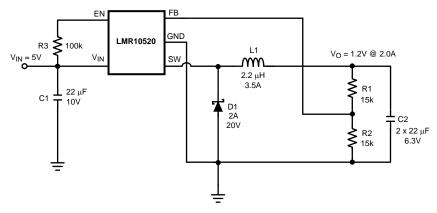
Figure 20. LMR10520x (1.6 MHz):  $V_{IN}$  = 5 V,  $V_{OUT}$  = 1.2 V at 2 A
