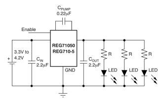
Figure 23. REG710 Circuit for Driving LEDs
