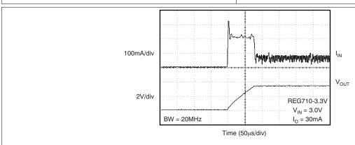
Figure 20. Input Current at Turn-On
