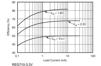
Figure 9. Efficiency vs Load Current
