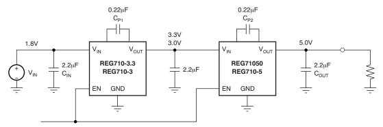
Figure 21. REG710 Circuit for Step-Up Operation From 1.8 V to 5 V With 10-mA Output Current
