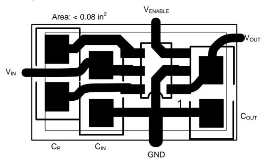
Figure 24. Suggested PCB Design for Minimum Ripple
