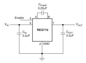
Figure 7. Typical Operating Circuit
