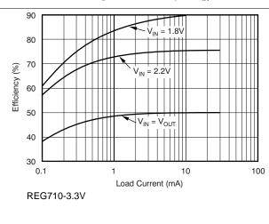
Figure 10. Efficiency vs Load Current
