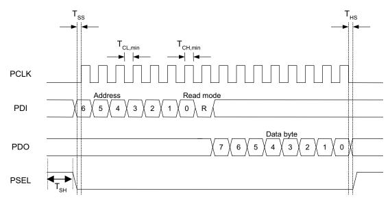
Figure 5-5. Configuration Registers Read Operation
