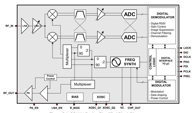
Figure 5-1. CC1021 Device Simplified Block Diagram
