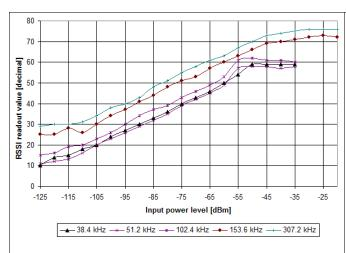
Figure 5-11. Typical RSSI Value vs Input Power for Different Channel Filter Bandwidths, 433 MHz
