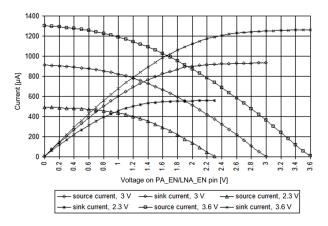
Figure 5-32. PA\_EN and LNA\_EN Pin Drive
