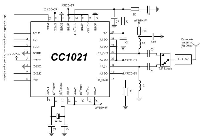
Figure 6-2. Alternative Application Circuit (Power Supply Decoupling Not Shown)
