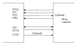
Figure 5-3. Microcontroller Interface
