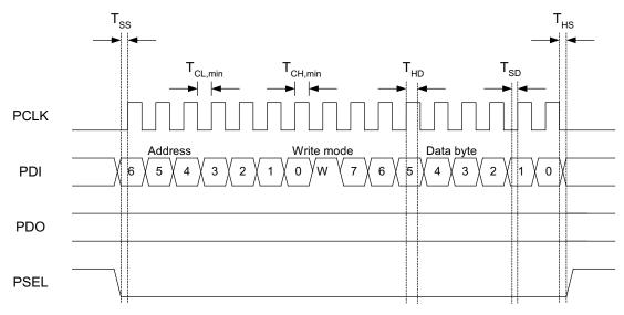
Figure 5-4. Configuration Registers Write Operation
