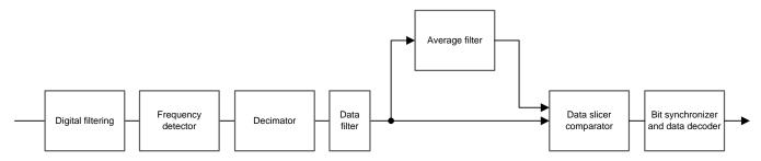
Figure 5-10. Demodulator Block Diagram
