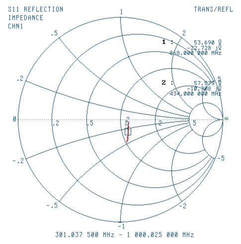
Figure 5-23. Typical LNA Input Impedance, 200 to 1000 MHz
