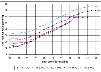
Figure 5-12. Typical RSSI Value vs Input Power for Different Channel Filter Bandwidths, 868 MHz
