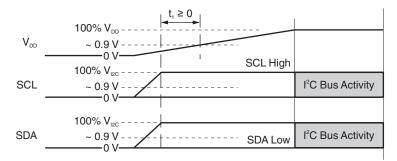
Figure 2. Power-On Sequence Timing Diagram
