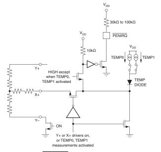
Figure 18. PENIRQ Functional Block Diagram
