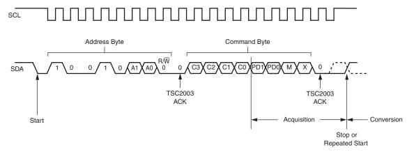
Figure 14. Complete I<sup>2</sup>C Serial Write Transmission
