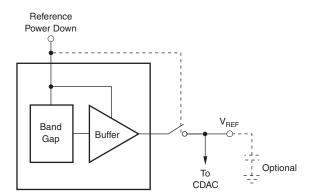
Figure 5. Simplified Diagram of the Internal Reference
