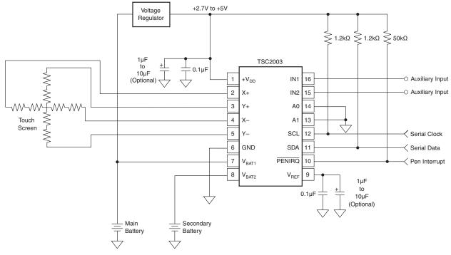
Figure 3. Basic Operation of the TSC2003
