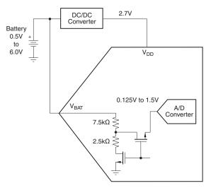
Figure 9. Battery Measurement Functional Block Diagram
