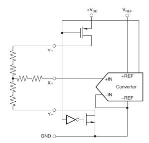
Figure 6. Simplified Diagram of Single-Ended Reference
