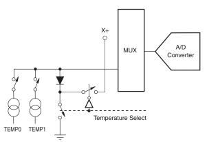
Figure 8. Temperature Measurement Mode Functional Block Diagram
