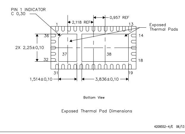
NOTE: All linear dimensions are in millimeters
