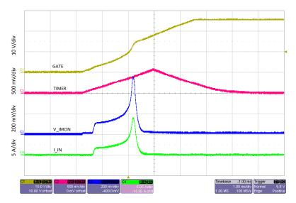
Figure 31. Inrush Mode at Hot-Swap Circuit Insertion
