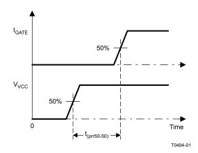
Figure 29. t<sub>prr50-50</sub> Timing Definition
