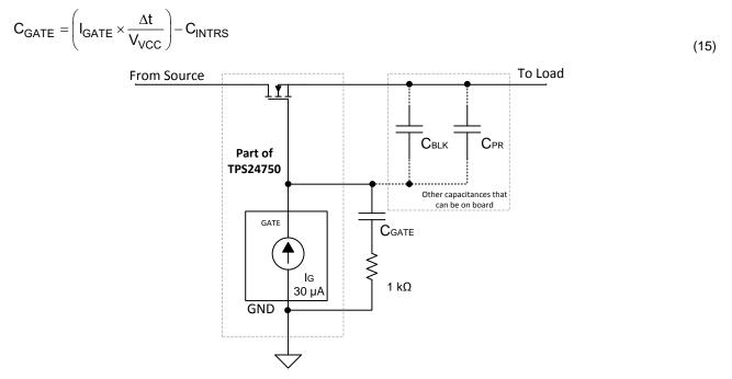
Figure 43. Gate Capacitor (dV/dt) Control Inrush Mode.
