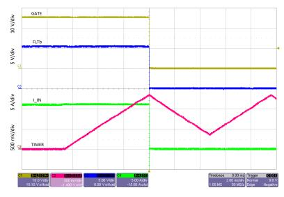
Figure 33. Circuit-Breaker Mode During Overload Condition
