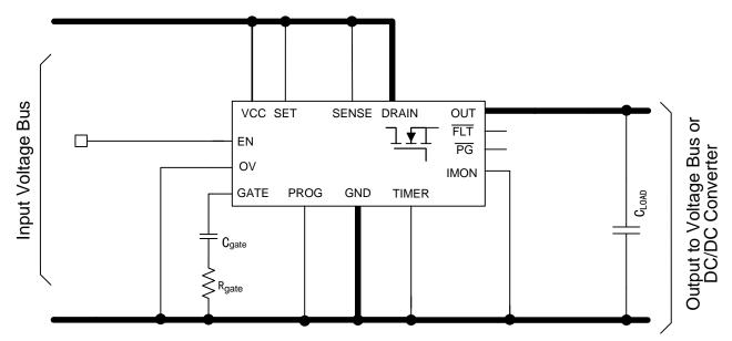
Figure 48. TPS2475x Configured as Simple 12-A Load Switch
