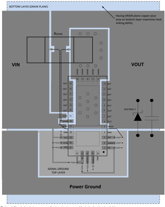
(1) Optional: Needed only to suppress the transients caused by inductive load switching.
