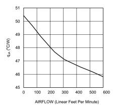
Figure 18. R<sub>OJA</sub> vs Airflow Speed (Jedec Board with 4 Vias)
