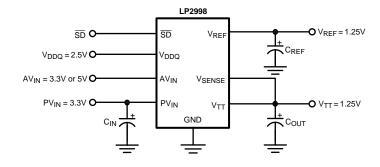
Figure 25. SSTL-2 Implementation with Higher Voltage Rails
