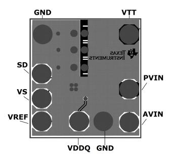
Figure 32. LP2998EVM SO PowerPAD Layout Example (Back)
