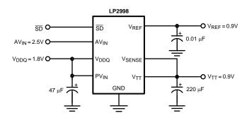
Figure 21. Recommended DDR-II Termination
