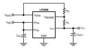
Figure 27. Decreasing VTT by Level Shifting
