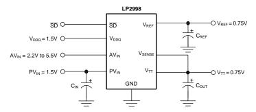
Figure 20. Recommended DDR-III Termination
