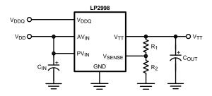
Figure 26. Increasing VTT by Level Shifting
