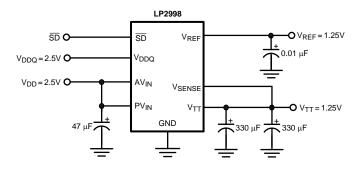
Figure 29. Typical SSTL-2 Application Circuit for Motherboards
