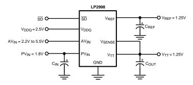
Figure 24. Lower Power Dissipation SSTL-2 Implementation
