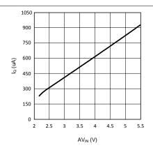
Figure 1.  $I_Q$  vs  $AV_{IN}$  In SD
