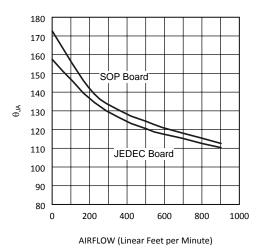
Figure 17. R<sub>0JA</sub> vs Airflow (SOIC-8)
