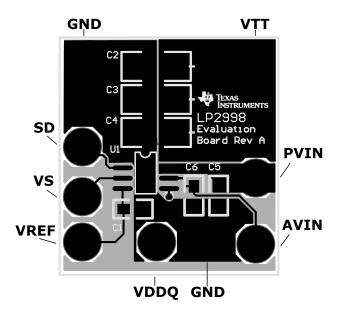
Figure 31. LP2998EVM SO PowerPAD Layout Example (Front)
