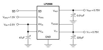
Figure 19. Typical Application Circuit
