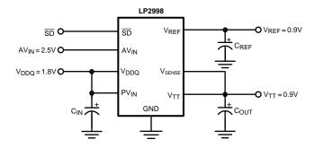
Figure 28. Typical SSTL-2 Application Circuit
