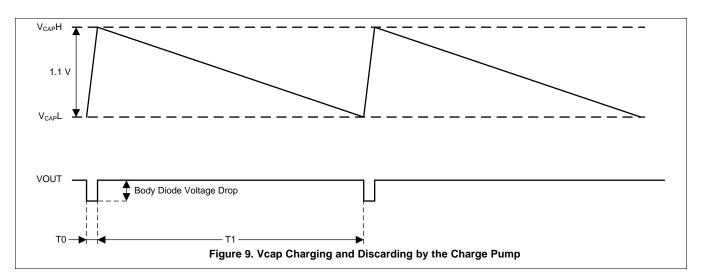
The Vcap current consumption is 1  $\mu$ A (typical) to drive the gate. The MOSFET OFF time (T0) and ON time (T1) can be calculated using the following expression
