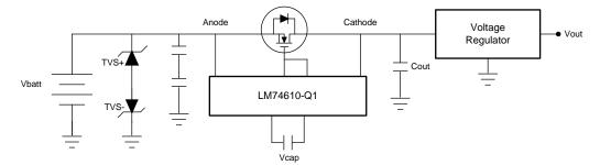
Figure 11. Typical System Application
