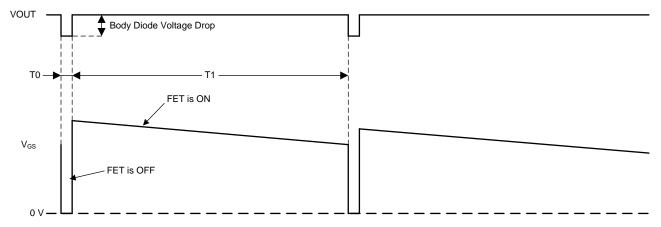
Figure 8. Output Voltage and V<sub>GS</sub>Operation at 1A Output Current
