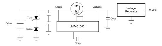
Figure 19. Typical Application without Positive Voltage Clamping
