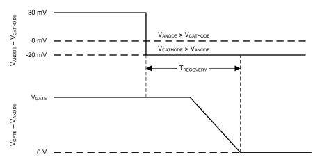
Figure 1. Gate Shut Down Timing in the Event of Reverse Polarity
