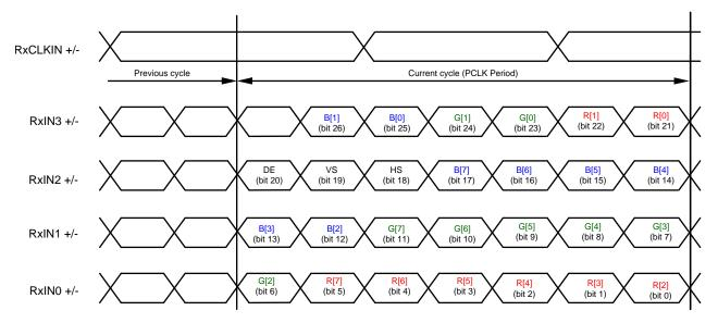
Figure 19. FPD-Link Mapping: LSBs on RxIN3 (MAPSEL=L)
