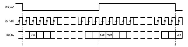
Figure 18. I<sup>2</sup>S Frame Timing Diagram
