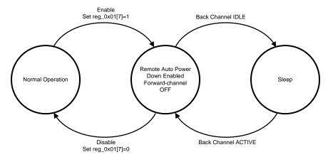
Figure 16. Remote Auto Power Down Sleep/Wake Cycle
