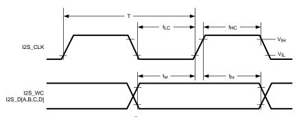
Figure 10. I<sup>2</sup>S Timing Diagram
