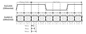
Figure 4. FPD-Link Input Strobe Position
