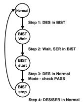
Figure 14. BIST Mode Flow Diagram
