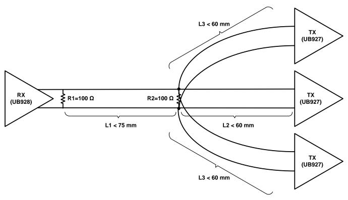
Figure 24. FPD-Link Fan-Out Electrical Requirements
