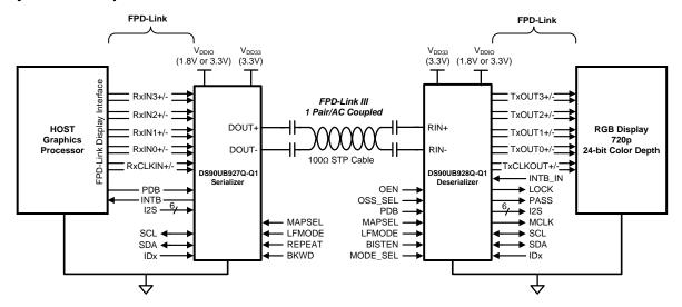
Figure 32. Color Display Application Diagram
