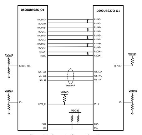
Figure 23. Repeater Connection Diagram
