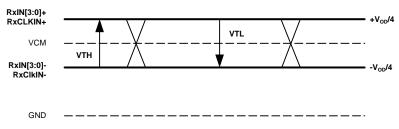
Figure 1. FPD-Link DC V<sub>TH</sub>/V<sub>TL</sub> Definition
