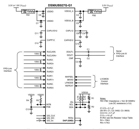
Figure 29. Color Display Typical Connection Diagram
