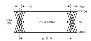
Figure 7. CML Serializer Output Jitter
