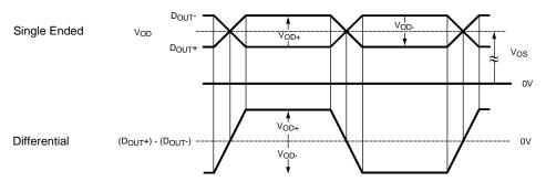
Figure 2. Serializer  $V_{\rm OD}$  DC Output
