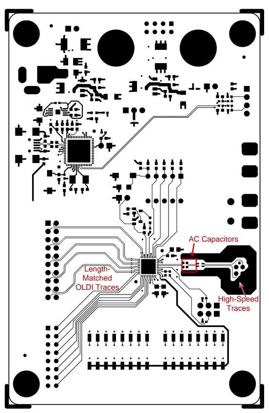
Figure 34. DS90UB927Q-Q1 Serializer Example Layout
