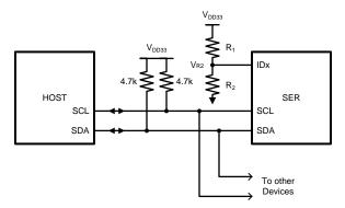
Figure 25. Serial Control Bus Connection
