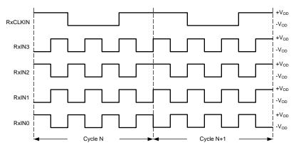
Figure 8. Checkerboard Data Pattern
