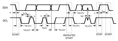
Figure 9. Serial Control Bus Timing Diagram
