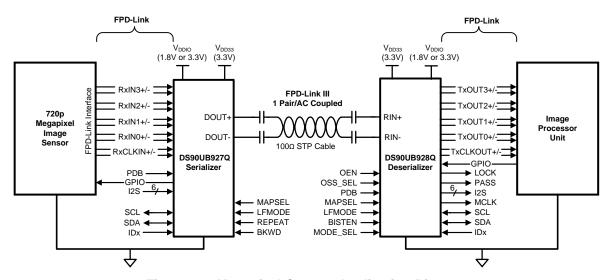
Figure 33. Megapixel Camera Application Diagram
