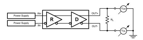
Figure 1. Differential Driver DC Test Circuit
