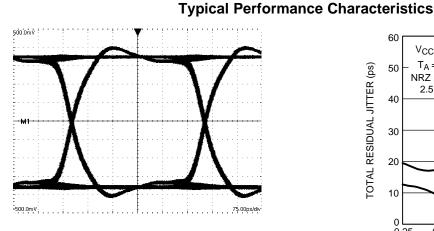
Figure 10. A 2.5 Gbps NRZ PRBS-7 Output Eye Diagram V:100 mV / DIV, H:75 ps / DIV
