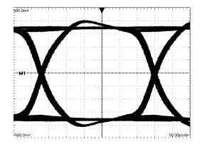
Figure 12. A 3.125 Gbps NRZ PRBS-7 Output Eye Diagram V:100 mV / DIV, H:50 ps / DIV
