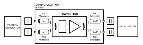
Figure 5. Jitter Measurements Test Circuit
