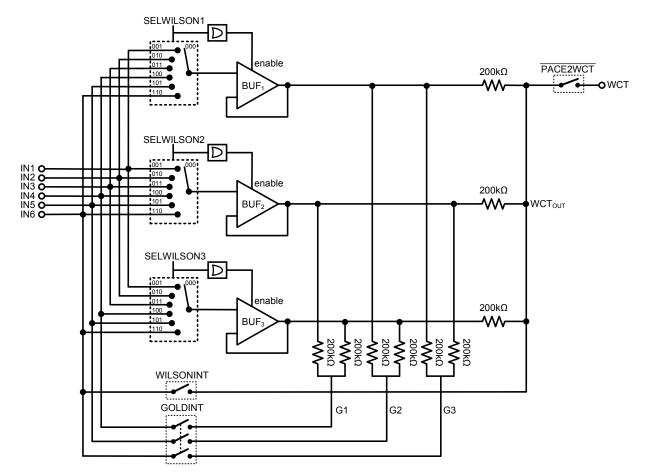
Figure 20. Wilson Reference Generator Circuit
