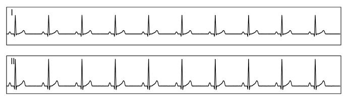
Figure 85. Single ADS1293 Device With an ECG Simulator, CH1 and CH2: ECG Signals
