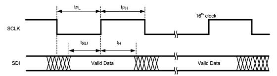
Figure 1. Write Timing Diagram
