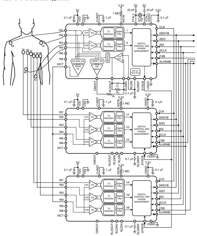
Figure 88. 8- or 12-Lead ECG Application
