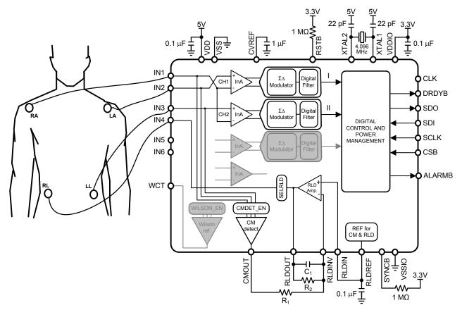
Figure 84. 3-Lead ECG Application
