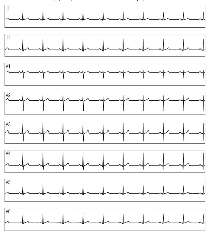
Figure 89. Three Synchornized ADS1293 Devices With an ECG Simulator: ECG Signals
