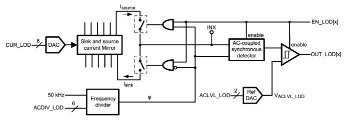
Figure 25. Simplified Analog AC Lead-Off Detect Block Diagram
