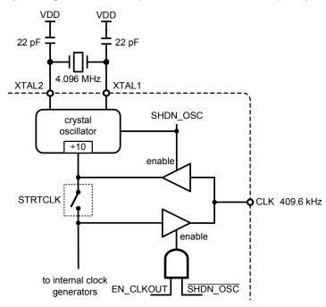
Figure 27. Block Diagram of the Clock
