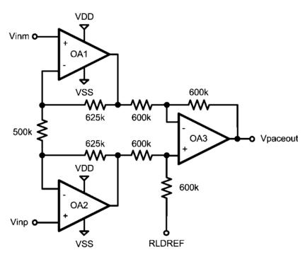
Figure 19. Analog Pace Channel Instrumentation Amplifier
