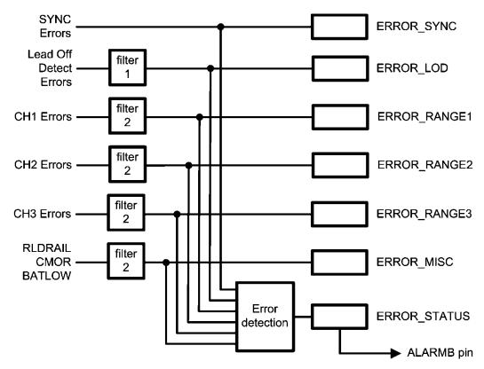
Figure 28. Graphical Illustration of Alarm Propagation
