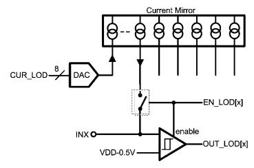
Figure 23. Simplified DC Lead-Off Detect Block Diagram
