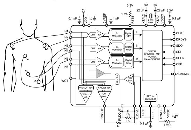
Figure 86. 5-Lead ECG Application
