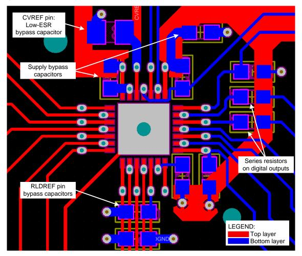
Figure 90. PCB Layout Example
