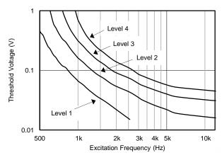
Figure 24. Analog AC Lead-Off Reference Levels
