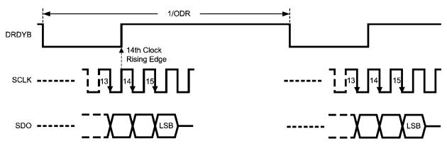
Figure 30. DRDYB Behavior for a Complete Read Operation
