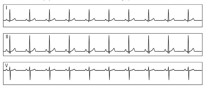
Figure 87. Single ADS1293 Device With an ECG Simulator, CH1, CH2, and CH3: ECG Signals
