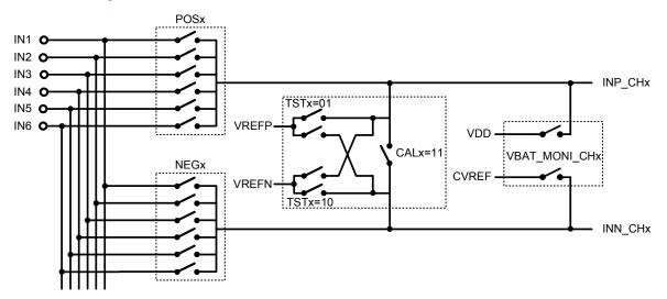
Figure 17. Flexible Routing Switch for Channel 1
