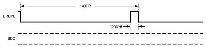
Figure 31. DRDYB Behavior for an Incomplete Read Operation
