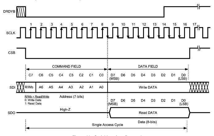
Figure 29. Serial Interface Protocol
