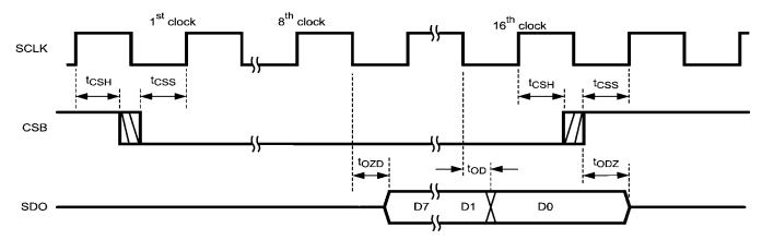
Figure 2. Read Timing Diagram
