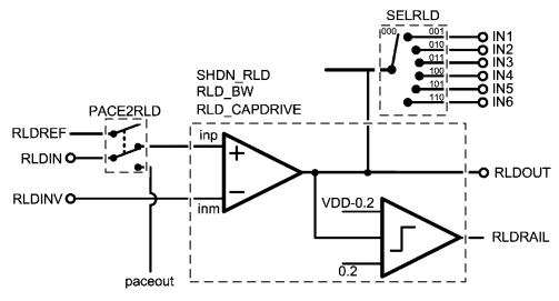
Figure 22. Right-Leg Drive Circuit
