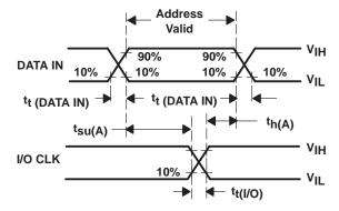
Figure 9. DATA IN Setup Voltage Waveforms
