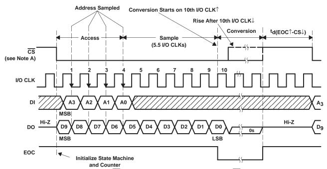
NOTE A: To minimize errors caused by noise at  $\overline{CS}$ , the internal circuitry waits for a setup time after  $\overline{CS} \downarrow$  before responding to control input signals. No attempt should be made to clock in input data until the minimum  $\overline{CS}$  setup time has elapsed.
