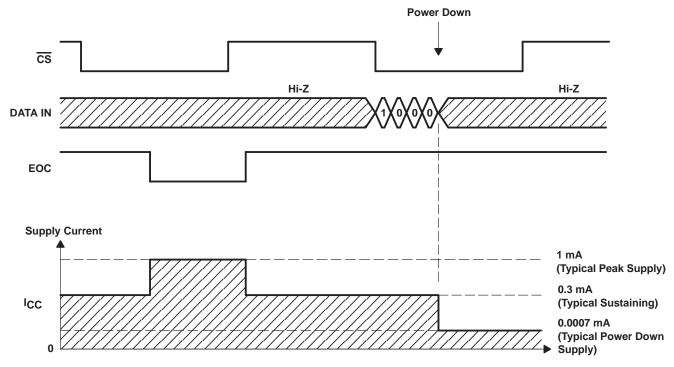
Figure 3. Typical Supply Current During Conversion/Power Down
