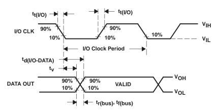
Figure 11. DATA OUT and I/O CLK Voltage Waveforms
