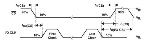
Figure 10. CS and I/O CLK Voltage Waveforms
