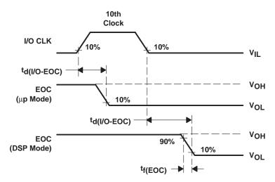
Figure 13. I/O CLK and EOC Voltage Waveforms
