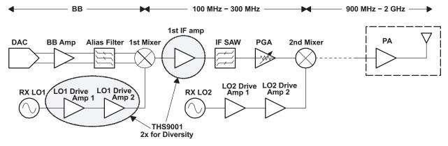
Figure 23. Example Dual Conversion Transmitter Architecture
