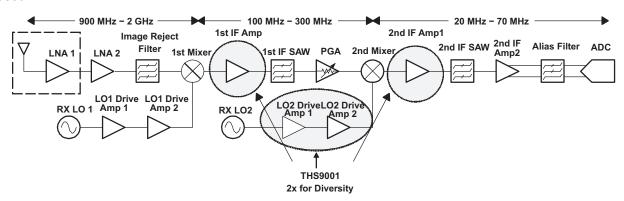
Figure 22. Example Dual Conversion Receiver Architecture
