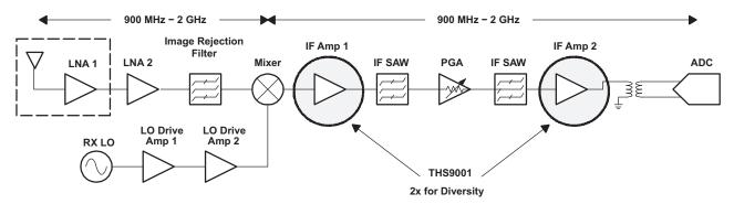
Figure 21. Example Single Conversion Receiver Architecture
