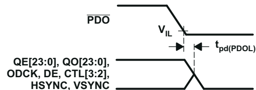
图 6-7. Delay From \overline{PDO} Low to Hi-Z Outputs
