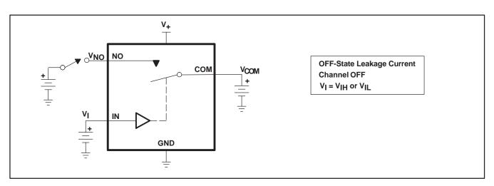
Figure 14. OFF-State Leakage Current (I<sub>COM(OFF)</sub>, I<sub>NO(OFF)</sub>)
