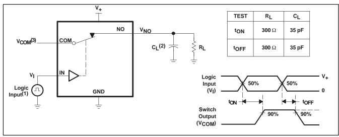
(1) All input pulses are supplied by generators having the following characteristics: PRR  $\leq$  10 MHz, Z<sub>O</sub> = 50  $\Omega$ , t<sub>f</sub> < 5 ns, t<sub>f</sub> < 5 ns.
