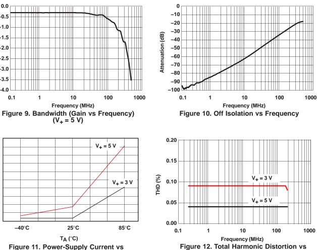
Figure 11. Power-Supply Current vs Temperature
