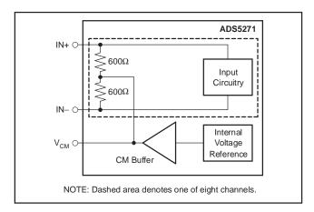
Figure 15. Analog Input Bias Circuitry
