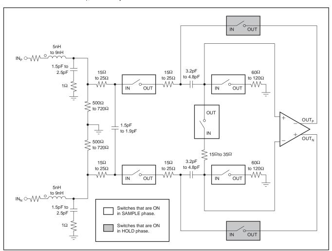
Figure 16. Overall Structure of the Sample-and-Hold Circuit
